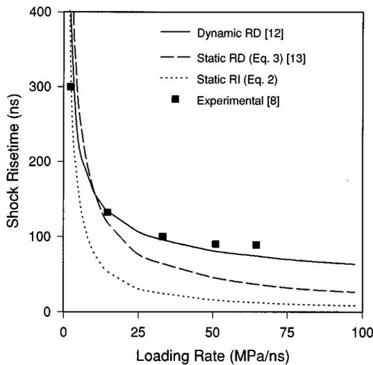
FIG. 1. The shock rise time of a porous aluminum-based material over a wide range of dynamic loading rates. The powder was initially at the ambient temperature, its porosity is 47% and a higher reference shear stress [ $\tau_0 = 175$  Mpa in Eq. (1)] was assumed to account for the 2 Al+Fe<sub>2</sub>O<sub>3</sub> powder mixture reported in the experiment (Ref. 8).
