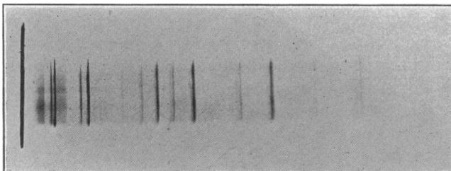
In order to determine accurately the value of the grating-constant, photographs were taken of the lines  $L\alpha_1$  of silver (first order) and  $K\alpha_1$  of copper (second order), using a vacuum spectrograph similar to that of Siegbahn,<sup>3</sup> and using his double exposure method.<sup>4</sup> As source for the X-radiation hot sparks<sup>5</sup> were used. The following data were obtained:
