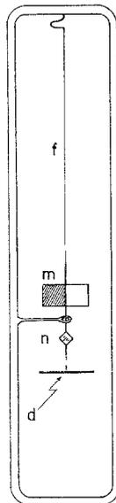
Fig. 1. The entire apparatus, except the aluminum foil vane, is made of fused quartz, fused together. Part  $d$ , whose moment of inertia is known, is removed after the period for torsional oscillation of the system has been measured. This permits a determination of the torsion constant of the fiber.
