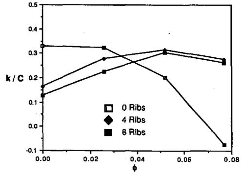
Fig. 7 Whirl ratio at 1000 rpm, no swirl
