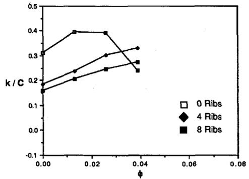
Fig. 6 Whirl ratio at 2000 rpm, no swirl
