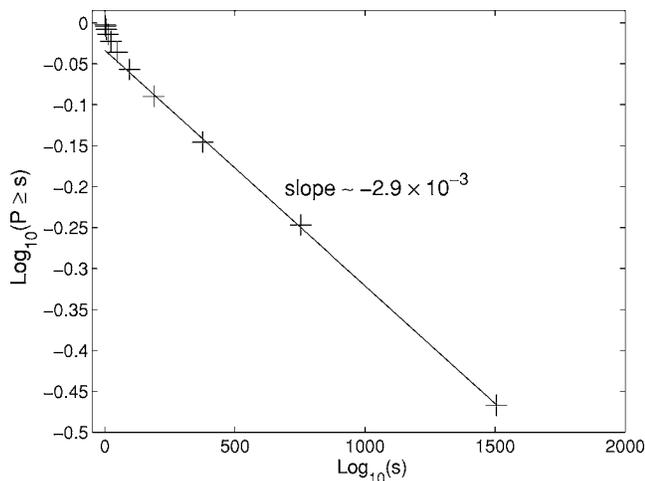
FIG. 9. HOT power law produced by a spark distribution with  $\psi(n) \sim n^{-0.4}$  on lattice with  $Z=3$ .
