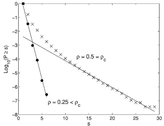
FIG. 4. Preferential growth. Cumulative number of strains  $P(\geq s)$  vs strain size  $s$  with  $Z=3$  and  $\rho=0.5$  (at the critical point) for  $\times$ 's, and  $\rho=0.25$  (below critical point) for the circles. Best fit lines are included in the log-linear plot to illustrate that the graphs are *not* power laws, and are in fact closer to exponential distributions. Note the difference in scale compared to Fig. 3.
