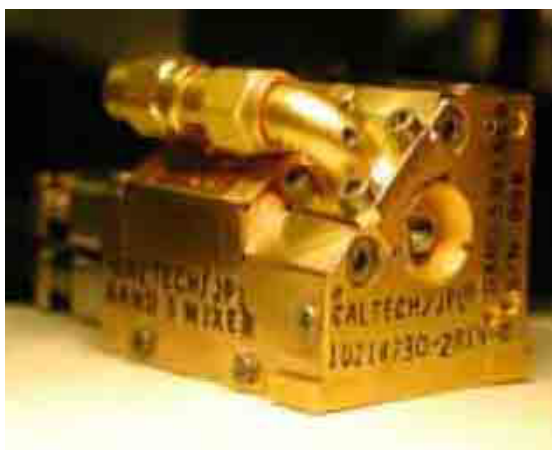
Figure 5. Twin-slot mixer evolution. Bottom Left : The first version, developed at U. Illinois in 1989 and tested at 500 GHz at Caltech in 1991. Top : The second version, flown on the KAO in 1993–95 for observations in the 500–800 GHz range. Bottom Right : The latest version, designed by A. Karpov at Caltech for use on Herschel/HIFI at 1.2 THz (Karpov et al. 2004).
