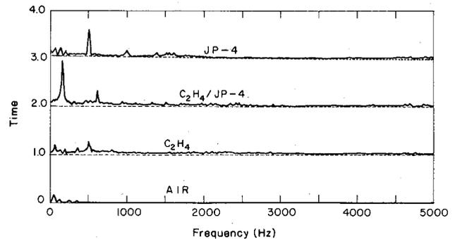
Fig. 5 Frequency content immediately downstream of shock.
