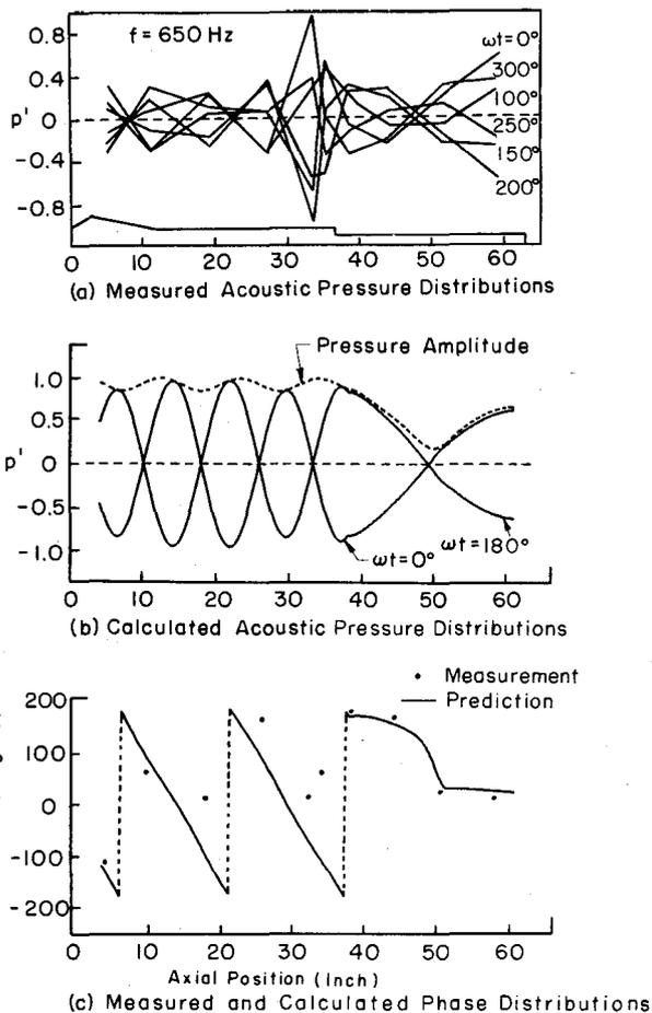
Fig. 9 Measured and calculated acoustic pressure amplitude and phase distributions (case 4,  $f = 650$  Hz, test D-163).
