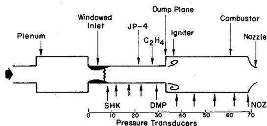
Fig. 1 Physical arrangement of laboratory ramjet engine.
