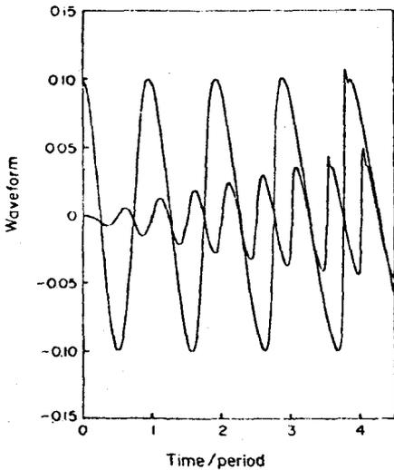
Fig. 2.5. Steepening of a standing wave in a pure gas according to the numerical analysis;  $f = 900$  Hz.
