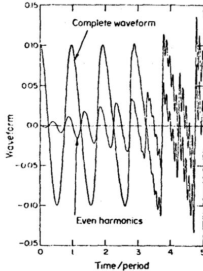
Fig. 2.6. Steepening of a standing wave in a pure gas according to the approximate analysis with ten modes accounted for;  $f = 900$  Hz.
