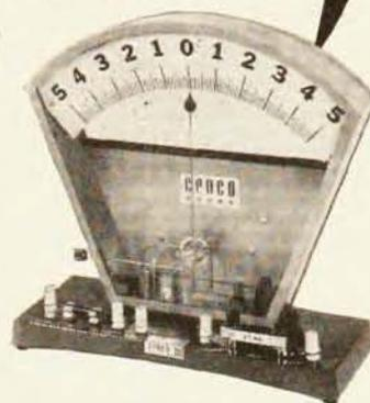
Now—a combination galvanometer, four-range voltmeter and four-range ammeter with figures and graduations on a large 17" scale that is plainly seen from both sides over any distance in the classroom. An accurate, versatile lecture meter with a modern, shielded movement. All parts and circuits clearly visible.
