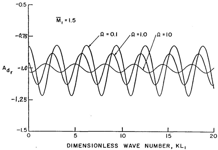
Fig. 3a. Real Part of Acoustic Admittance Function at the Inlet Side of the Dump Plane ( $x = 0_-$ )
