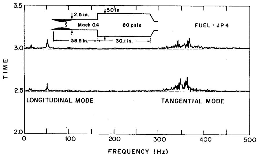
Fig. 2. Frequency Content of Pressure Oscillations in a Laboratory Ramjet Combustor
