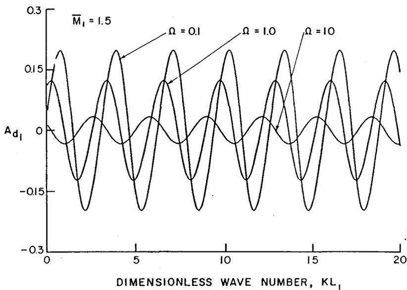
Fig. 3b. Imaginary Part of Acoustic Admittance Function at the Inlet Side of the Dump Plane ( $x = 0_-$ )
