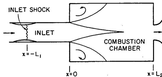
Fig. 1. Schematic Diagram of Ramjet Engine
