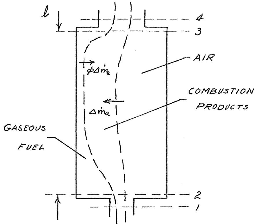
Figure 1. One-Dimensional Model for Room Combustion and Convection.
