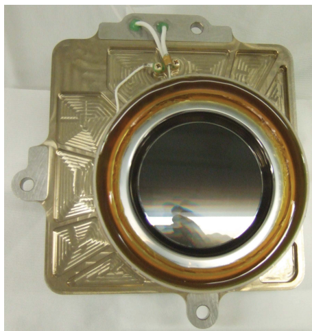
Figure 1. FIREBALL NUV Detector: Legacy GALEX NUV microchannel plate detector used by the FIREBALL spectrograph.
