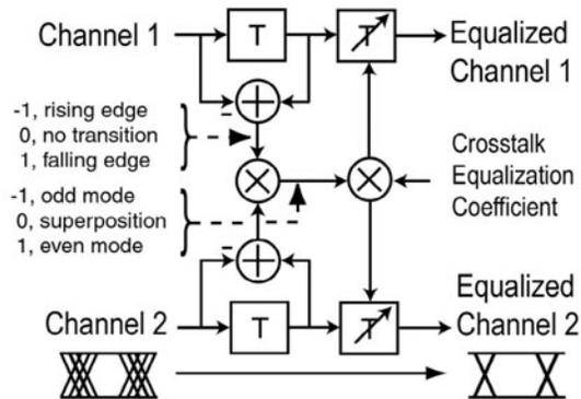
Fig. 2. Schematic of a two-channel crosstalk-induced jitter cancellation.
