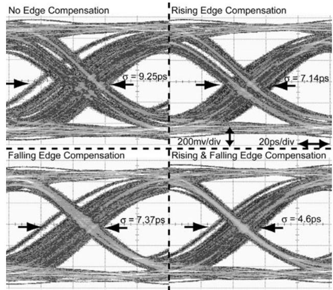
Fig. 7. Eye diagrams for DDJ compensation of different edges at 10Gb/s.
