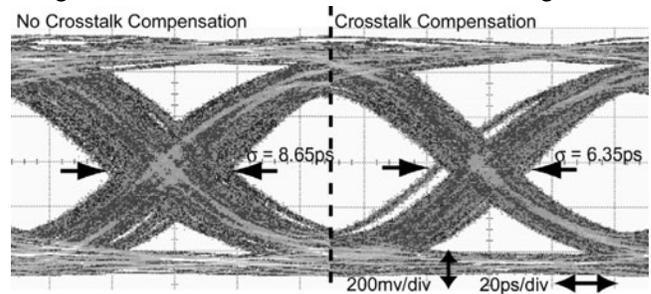
Fig. 5. Data eyes at 10Gb/s before and after equalization.
