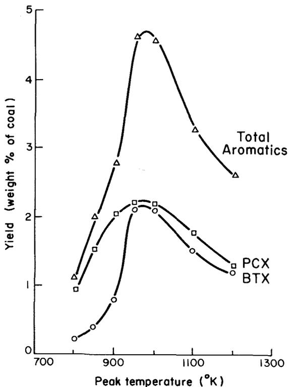
Fig. 7.6. Yield of single ring aromatic products vs. peak temperature for hydroypyrolysis of a bituminous coal at 150 bar pressure and 11s hydrogenolysis residence time (source: ref. 144).
