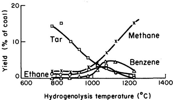
Fig. 7.8. Product yields vs. hydrogenolysis temperature for a bituminous coal at heating rate  $10^4$  K/s, peak hydrolysis temperature  $750^{\circ}$ K and hydrogen pressure 100 bar (source: ref. 144).
