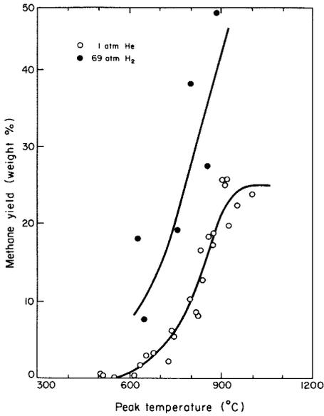
Fig. 7.3. Methane yield vs peak temperature for pyrolysis and hydrolysis of a bituminous coal "Pittsburgh No. 8" (source: ref. 63).
