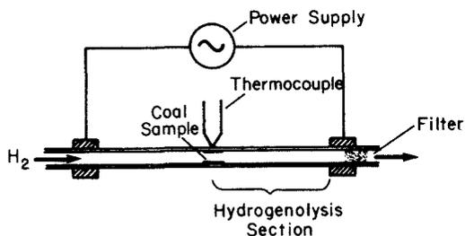
Fig. 7.10. Modified captive sample reactor for coal hydrolysis (source: ref. 145).
