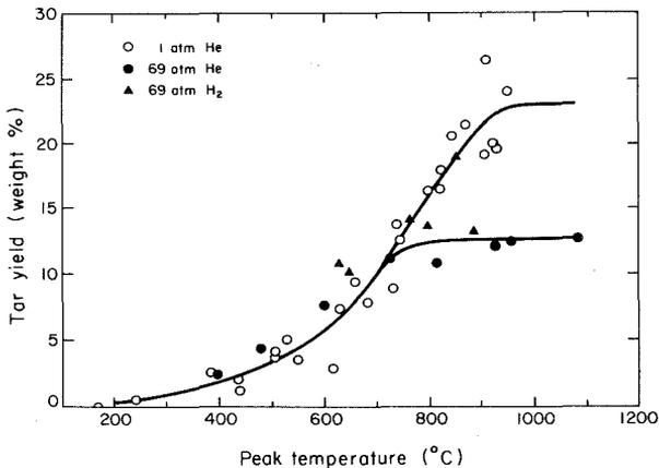
Fig. 7.2. Tar yield vs. peak temperature for pyrolysis and hydro-pyrolysis of a bituminous coal "Pittsburgh No. 8" (source: ref. 63).
