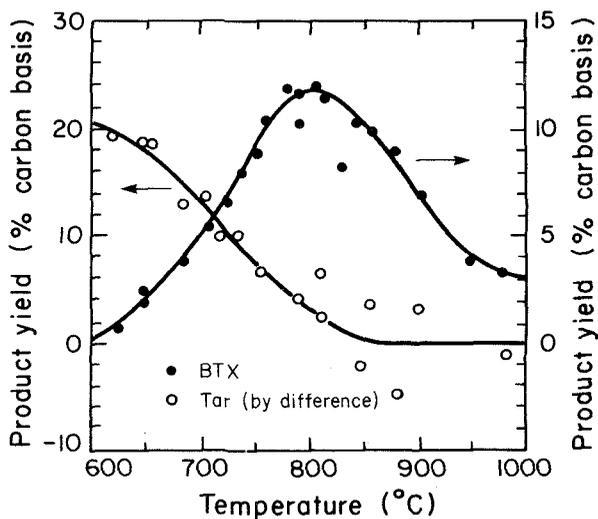
Fig. 7.12. Yields of BTX and tar (by difference) vs. temperature for hydropyrolysis of a bituminous coal "Illinois No. 6" at 100 atm H<sub>2</sub>, 650°C/s heating rate and 0.6s hydrogenolysis time (source: ref. 146).
