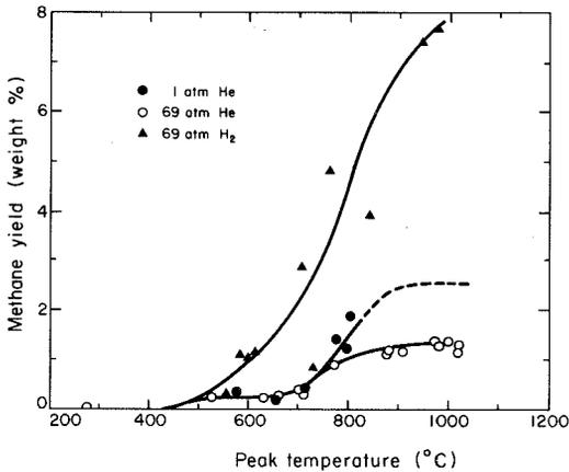
Fig. 7.4. Methane yield vs. peak temperature for pyrolysis and hydrolysis of a lignite (source: ref. 63).
