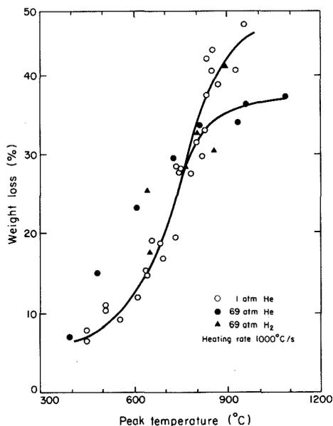
Fig. 7.1. Weight loss vs. peak temperature for pyrolysis and hydro-pyrolysis of a bituminous coal "Pittsburgh No. 8 (source: ref. 63).
