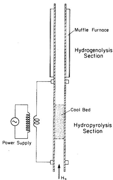
Fig. 7.5. Schematic of two-segment hydropyrolysis reactor used by Finn et al. (ref. 144).
