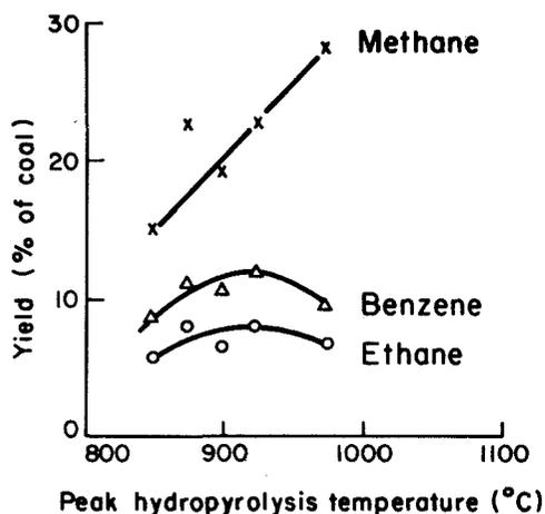
Fig. 7.9. Product yields vs. peak hydrolysis temperature for a bituminous coal at heating rate  $5^{\circ}\text{K/s}$ , hydrolysis temperature  $1123^{\circ}\text{K}$  and hydrogen pressure 150 bar (source: ref. 144).
