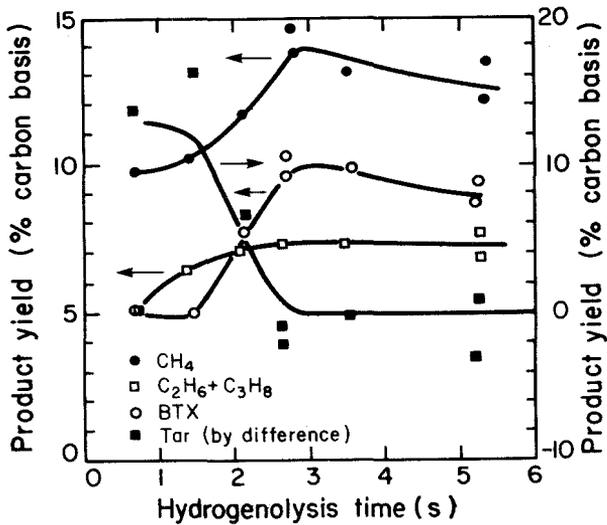
Fig. 7.13. Product yields vs. hydrogenolysis time for hydropyrolysis of a bituminous coal "Illinois No. 6" at 700°C, 100 atm H<sub>2</sub> and 650°C/s heating time (source: ref. 146).
