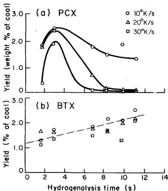
Fig. 7.7. Yield of BTX and PCX vs. hydrogenolysis time at different heating rates for hydrolysis of a bituminous coal at 150 bar pressure and 1000°K peak temperature (source: ref. 144).
