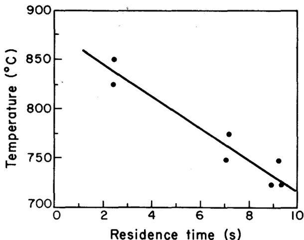
Fig. 7.14. Locus of maximum BTX yield for hydropyrolysis of lignite at 2500 psia  $H_2$  (source: ref. 147).
