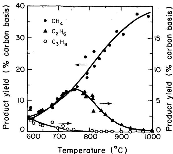
Fig. 7.11 Yield of gaseous hydrocarbons vs. temperature for hydropyrolysis of a bituminous coal "Illinois No. 6" at 100 atm H<sub>2</sub> and 0.6s hydrogenolysis time (source: ref. 146).
