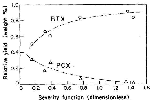
Fig. 7.17. Relative yields of BTX and PCX in the liquid products as a function of severity for the hydropyrolysis of a lignite at 2000 psia  $H_2$  (source: ref. 148).
