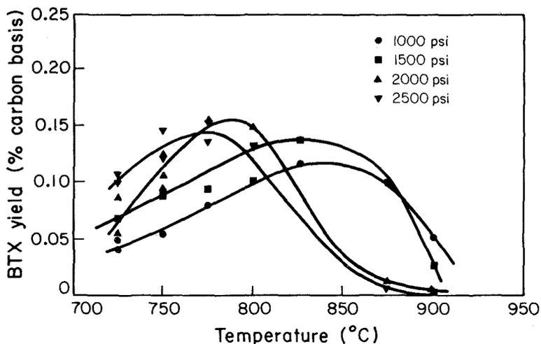
Fig. 7.16. Maximum BTX yield vs. temperature for hydropyrolysis of a subbituminous coal at various hydrogen pressures (source: ref. 147).
