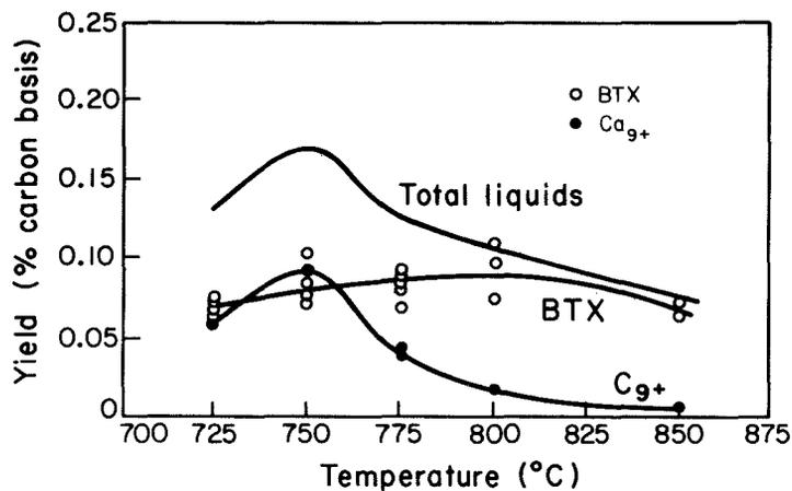
Fig. 7.15. Maximum yields of BTX and  $C_{9+}$  liquids vs. temperature for hydropyrolysis of lignite at 2000 psia  $H_2$  (source: ref. 147).
