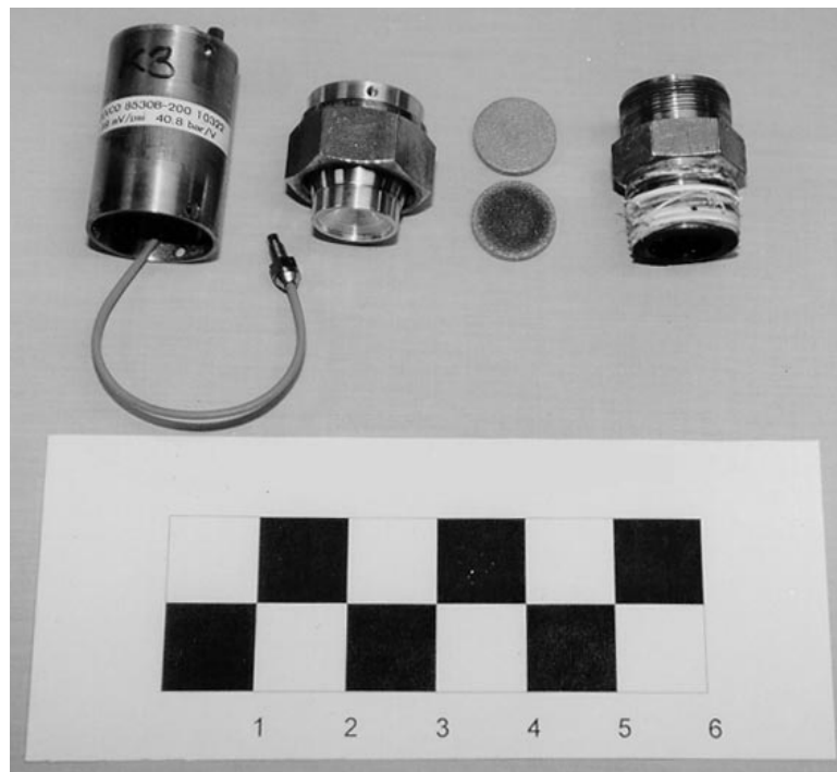
Figure 2.21: Endevco quasi-static pressure gauge with housing.
