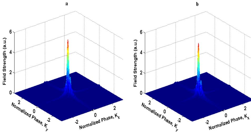
Fig. 5. The 2D spatial Fourier transform of the magnetic field above the slab waveguide for the case of a slab waveguide coupled to: (a) a PCW as shown in Fig. 1 and (b) a perfect PC structure with  $r=0.3a$  every where and no defect as shown in Fig. 4. All properties of the structures in (a) and (b) are the same as those in the caption of Fig. 1 and Fig. 4, respectively.
