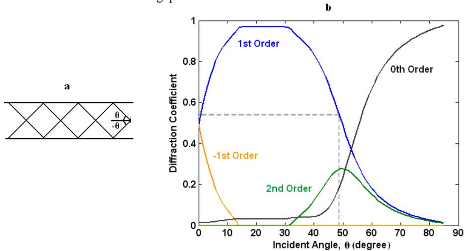
Fig. 6. (a) The slab waveguide with  $TM_0$  mode as a superposition of two plane waves with incident angles of  $\theta = \pm 48.8^\circ$ . (b) The variation of the approximate relative strength of different diffraction orders with the incident angle for the structure in Fig. 4 calculated using the grating theory with approximations described in the text. The dashed line corresponds to the incident angle of  $48.8^\circ$ .
