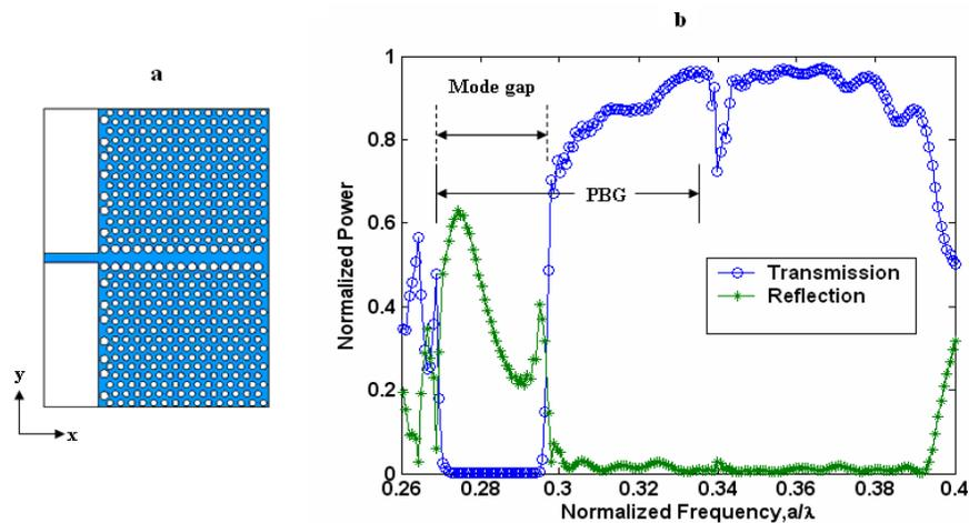
Fig. 7. (a) A slab waveguide coupled to a PCW with uniform perturbation of  $\pm 0.2a$  in the center of air holes in the  $y$  direction next to the interface. (b) The transmission and reflection spectra of the power coupled from slab waveguide to this perturbed structure with  $x=x_0=40$ ,  $x=x_1=450$ , and  $x=x_2=20$ .
