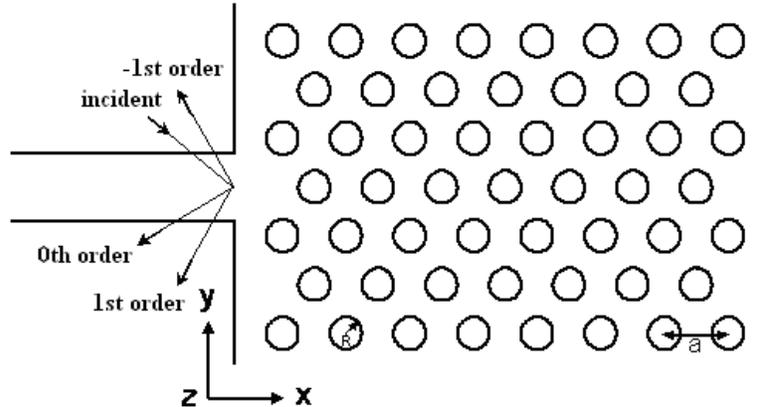
Fig. 4. A slab waveguide coupled to a perfect PC structure with  $r=0.3a$  (and  $a=24$ ). Different diffracted orders are shown in the figure. Other properties of the structure are similar to those summarized in the captions of Fig. 1.
