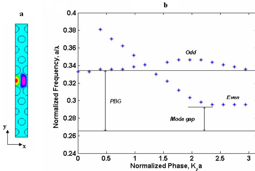
Fig. 2. (a) One period of the PCW with the magnetic field pattern of the fundamental even TM mode. (b) Dispersion diagram of the first two TM modes of the PCW in part (a). The odd mode exists outside the PBG and only the even mode remains inside the bandgap. The mode gap corresponds to the frequencies within the PBG with no allowed guided mode.
