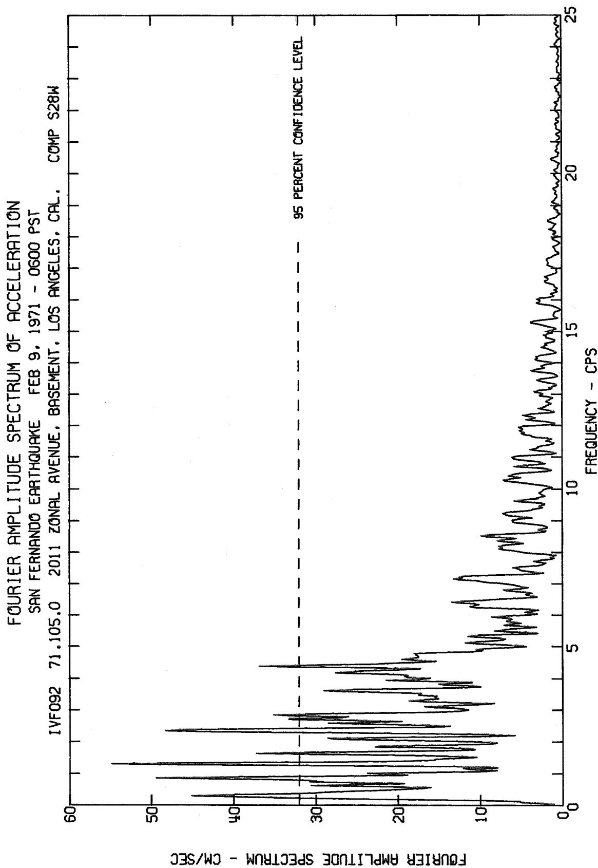
FOURIER AMPLITUDE SPECTRUM OF ACCELERATION
