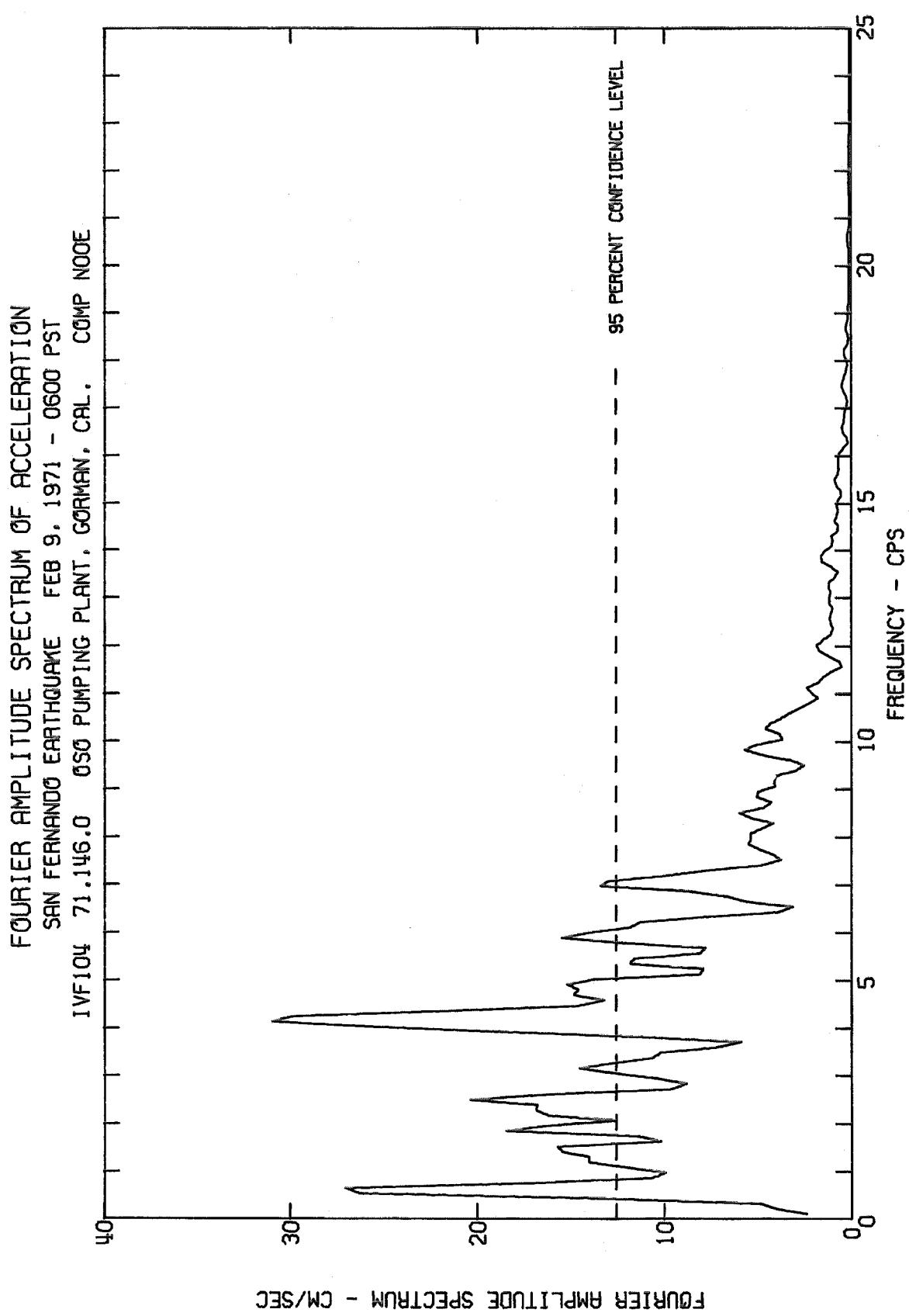
FOURIER AMPLITUDE SPECTRUM OF ACCELERATION
