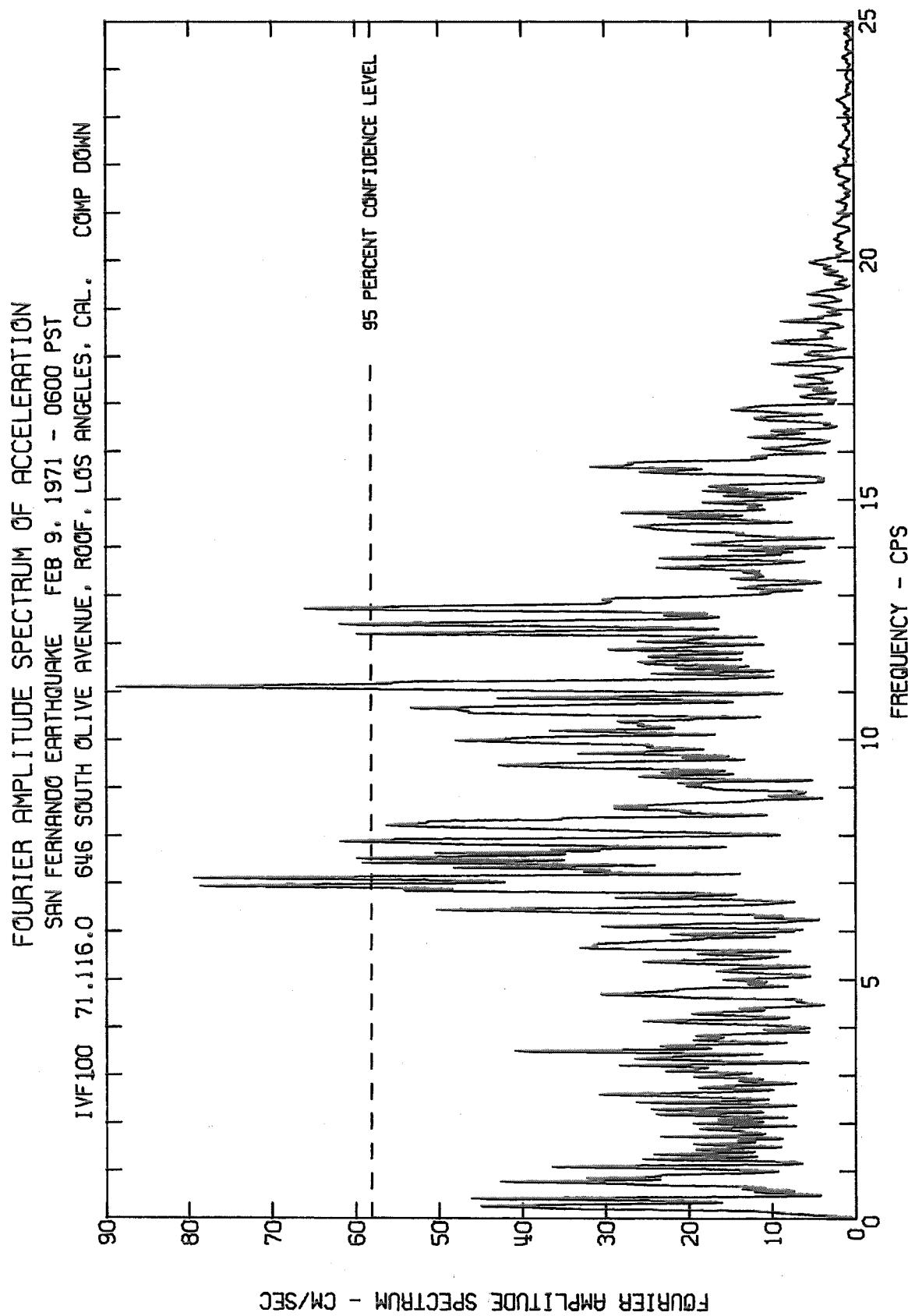
FOURIER AMPLITUDE SPECTRUM OF ACCELERATION
