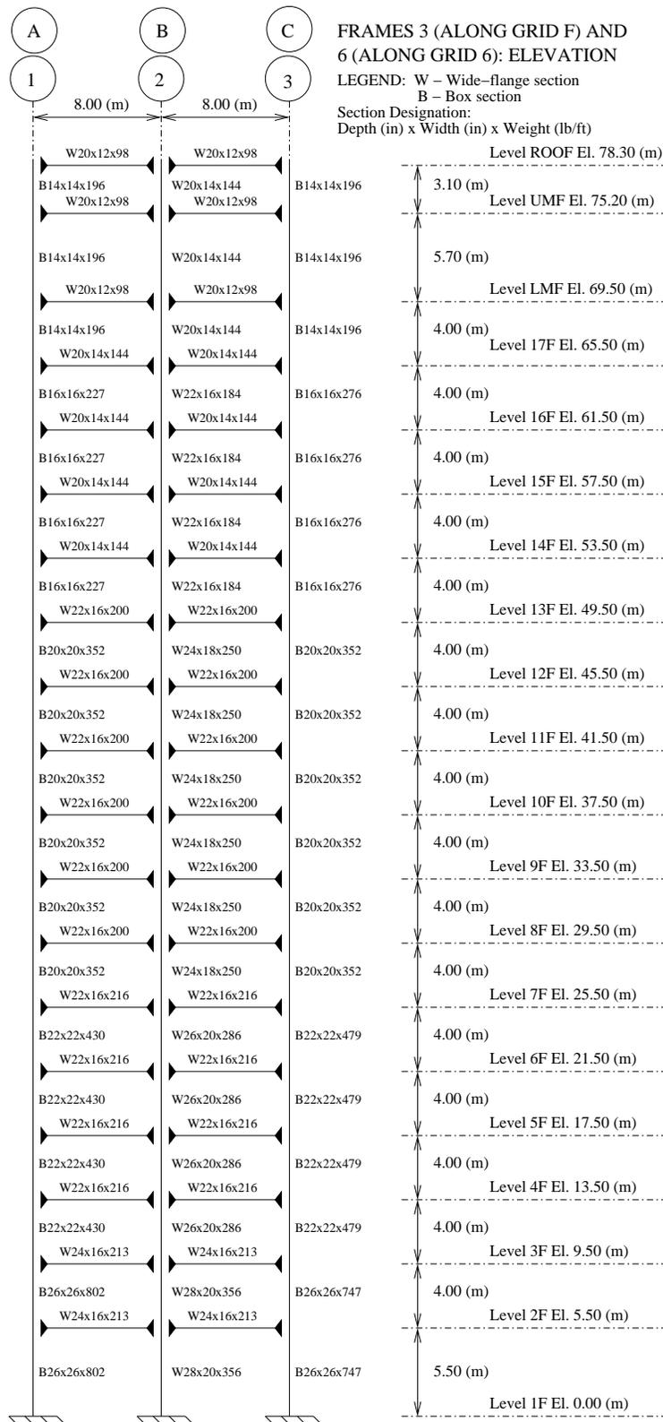
Figure C.12: Frames 3 & 6 Elevation: Building 2A
