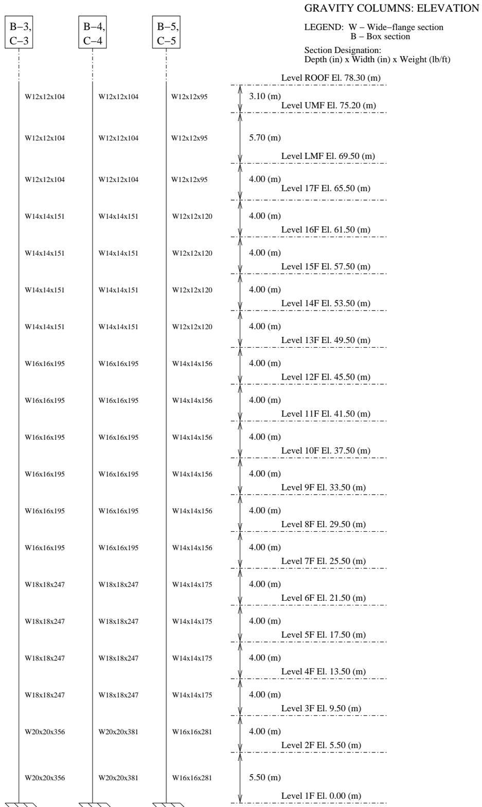
Figure C.21: Gravity Columns Elevation: Building 3A
