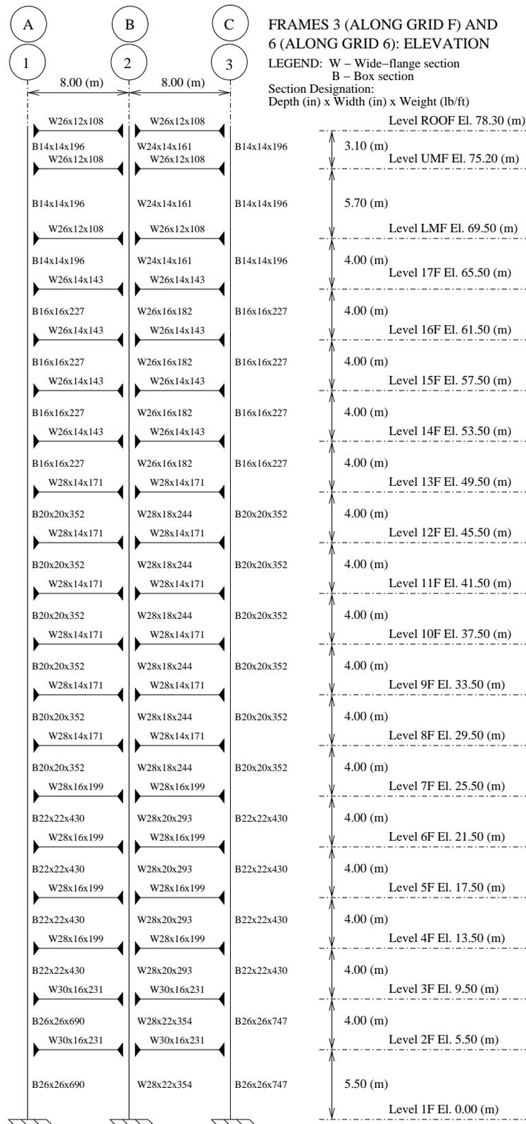
Figure C.8: Frames 3 & 6 Elevation: Building 2
