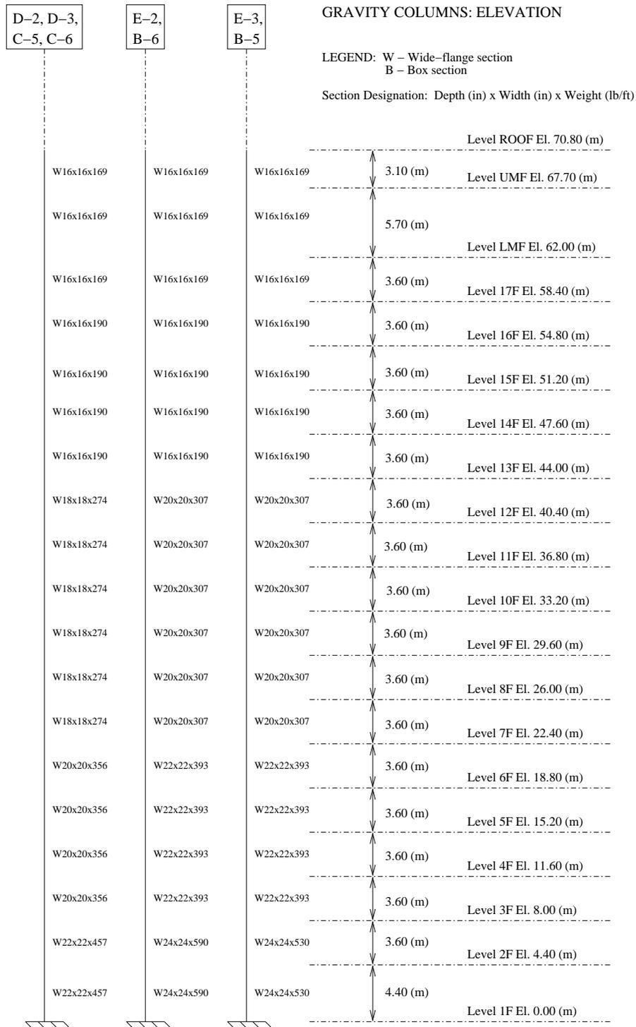
Figure C.5: Gravity Columns Elevation: Building 1
