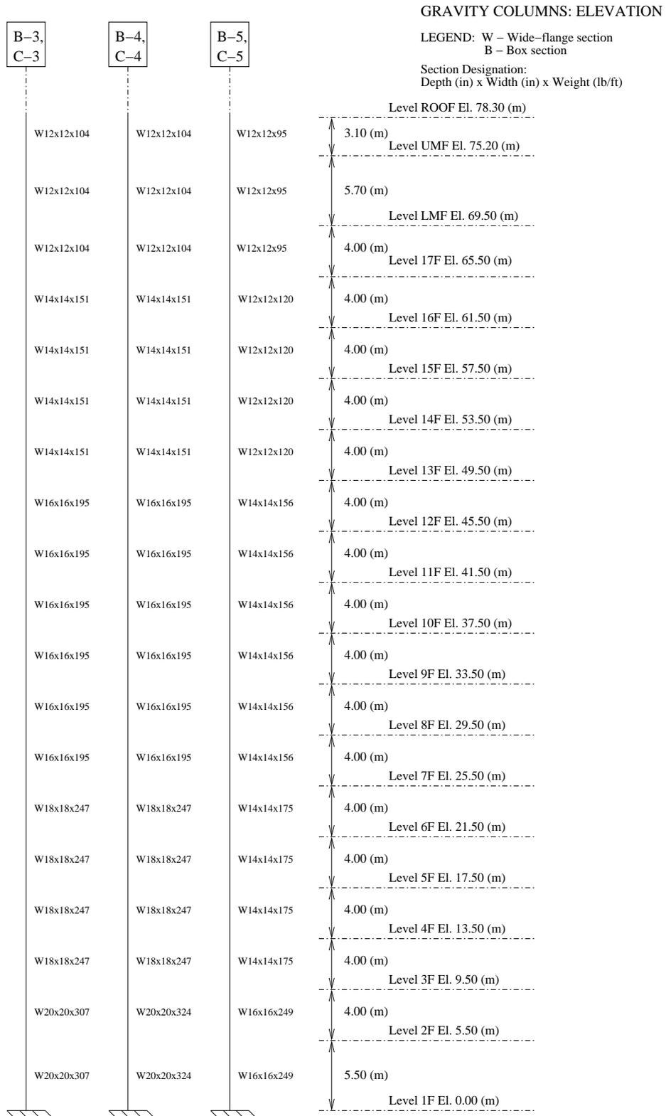
Figure C.17: Gravity Columns Elevation: Building 3
