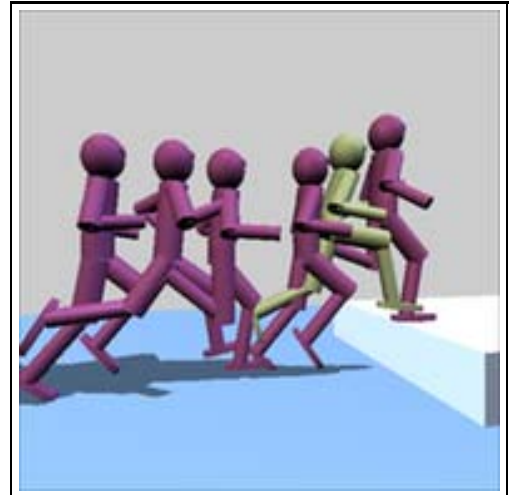
Figure 12. Optimizing the animation from the same keyframes, the foot does not pass through the step. The soft constraints have lifted the foot out of the way.
