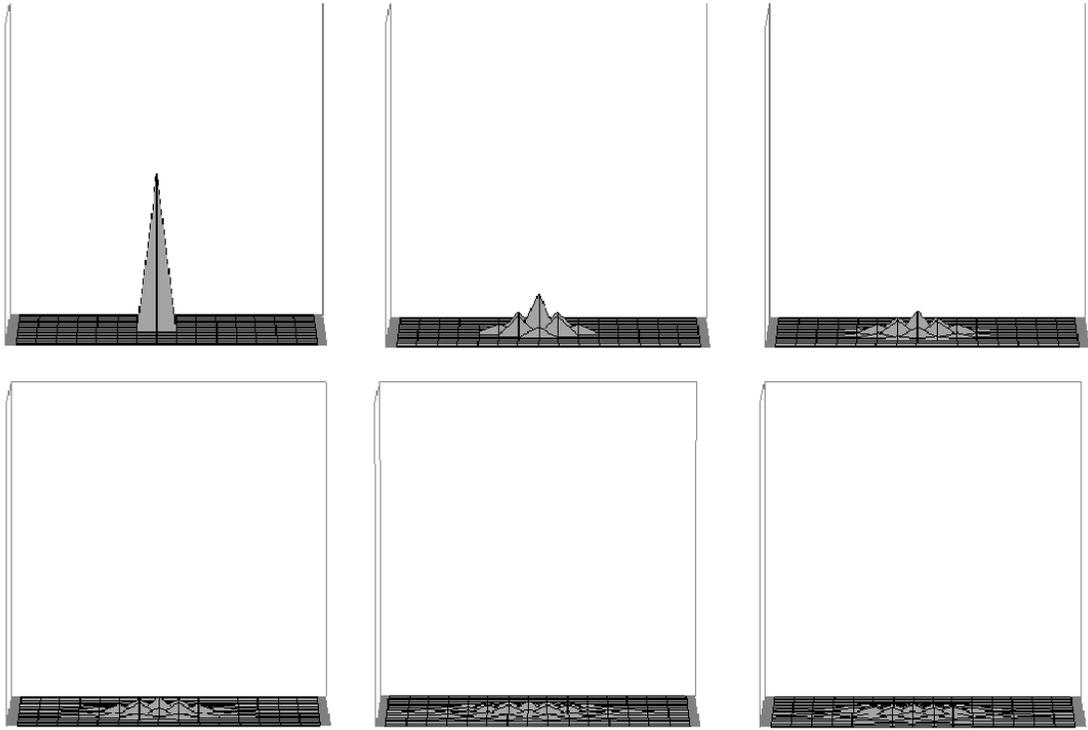
Figure 3.3: *Point disturbance under equation 3.5 shows monotone convergence.*
