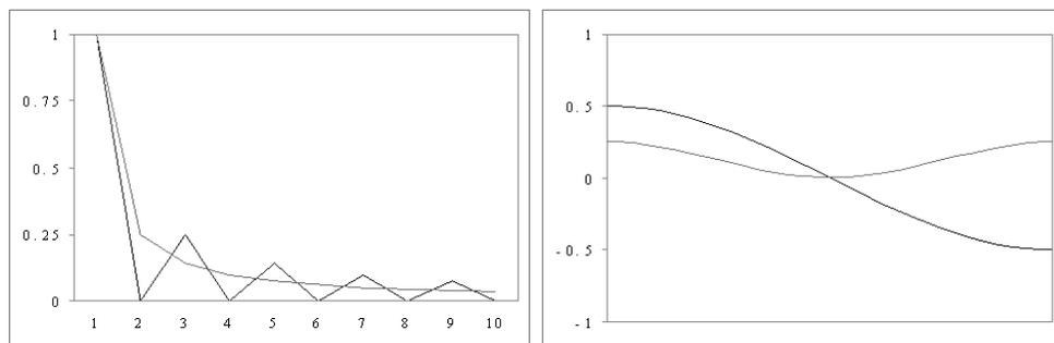
Figure 3.4: *Left, height of the point disturbance over 10 iterates of equations 3.2 and 3.5. Equation 3.2 shows oscillation while algorithm 3.5 converges monotonically. Right, eigenvalue  $\lambda_{i,8}$  for  $n = 16$  of iteration matrices  $A$  and  $AA$  corresponding to the two equations.  $A$  has mixed eigenvalues while  $AA$  is positive definite.*
