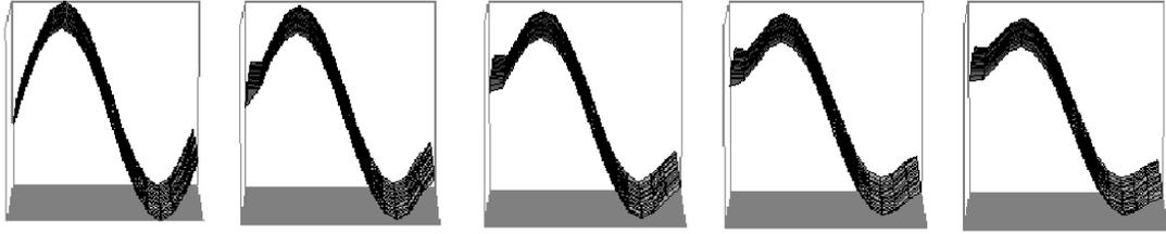
Figure 3.1: The “Achilles heel” of equations 3.2 and 3.5. This sinusoidal disturbance is the eigenvector  $\vec{X}_{i,j}$  that corresponds to the most slowly converging eigenvalue  $\lambda_{i,j}$  of equation (3.2). The standard iterations cannot converge this disturbance effectively.
