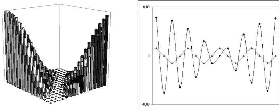
Figure 2.1: *Characteristics of the  $16 \times 16$  Laplacian matrix of a regular mesh. Left, the complete eigenvalue spectrum. Right, two representative eigenvectors. The eigenvector with the larger variation is the Fiedler vector.*
