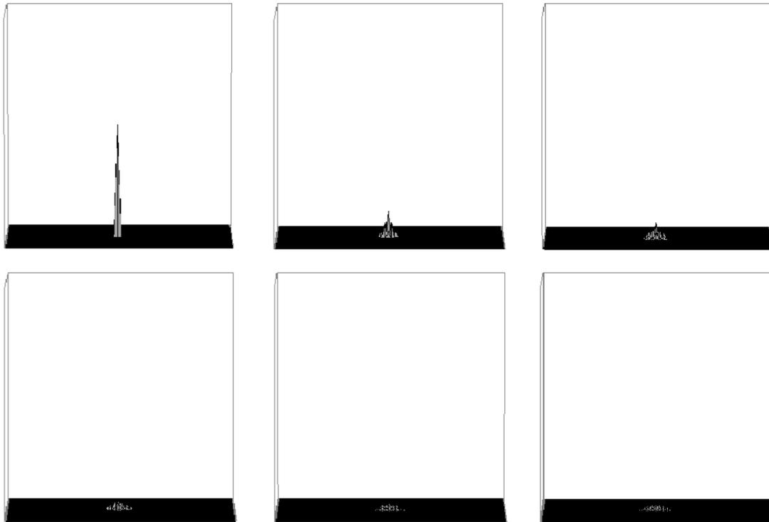
Figure 3.5: *Convergence of a problem on a  $64 \times 64$  grid of 4096 unknowns. The height of the initial disturbance is the same in this series as in figure 3.2 affirming the conclusion of the Scalability Theorem.*
