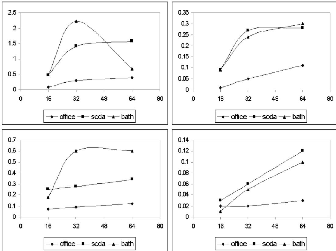
Figure 4.6: Comparison of effective imbalance  $\epsilon$  with and without dynamic load balancing by algorithm 1, for the three images in table 4.2. Clockwise from upper left: naive method only; naive method followed by algorithm 1; scatter method followed by algorithm 1; scatter method alone. In several cases the initial imbalance seems to correlate with the effective imbalance under algorithm 1.
