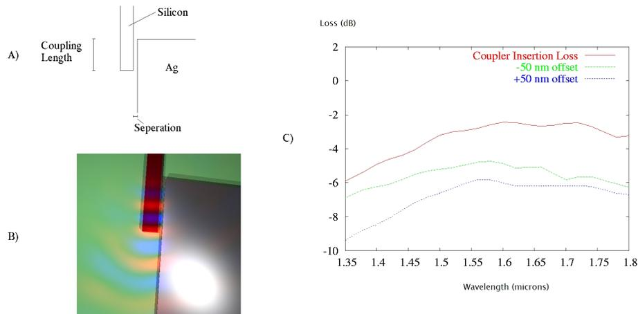
Fig. 2. (a) shows a diagram of the layout of the dielectric plasmon coupling device. A rendering of a simulation is shown in (b), while (c) shows the simulated insertion loss for the coupling device in dB vs wavelength in  $\mu\text{m}$ . Also shown are the insertion losses when the coupling device separation is increased or decreased by 50 nm, as might happen due to misalignment in fabrication.
