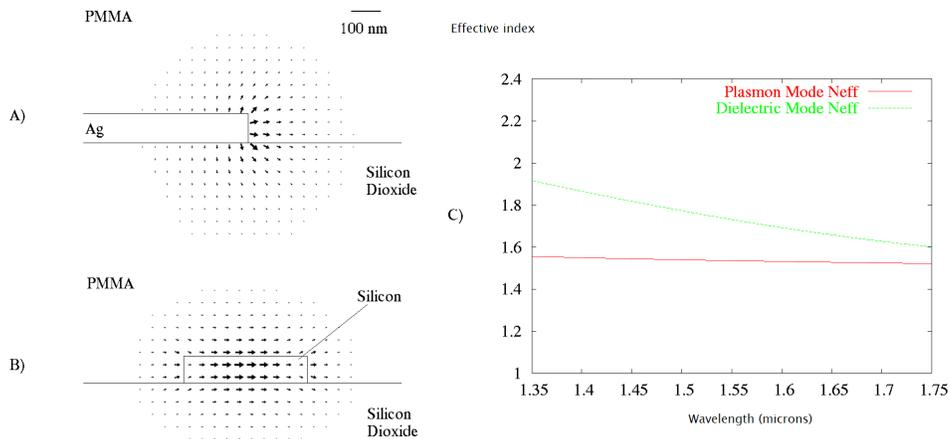
Fig. 1. In A) and B) the E field vector components are rendered for the plasmon and silicon waveguides used in our study. C) shows the dispersion diagrams of both modes.
