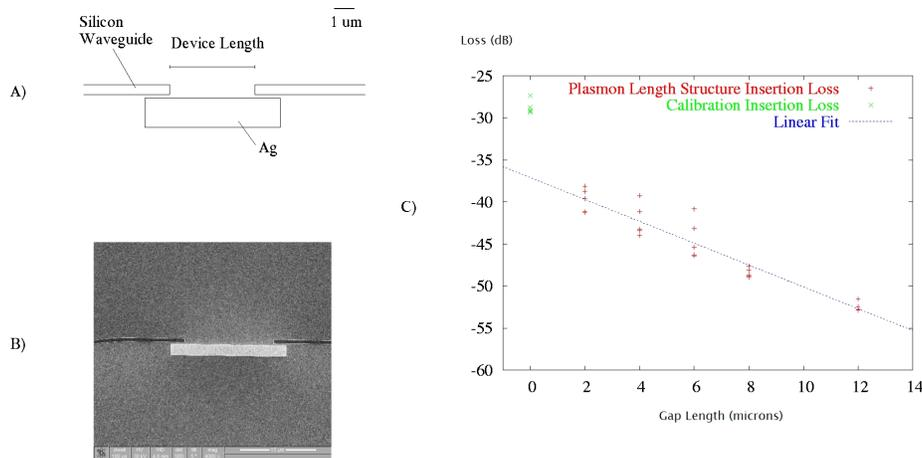
Fig. 3. (a) shows a diagram of the layout of a plasmon waveguide length device, and (b) shows an SEM image of a fabricated device. (c) shows the scatter plot and fitted line, as well as a scatter plot of the 5 best calibration insertion loss structures for contrast. The axes are fiber to fiber insertion loss in dB versus plasmon waveguide length in  $\mu\text{m}$ .
