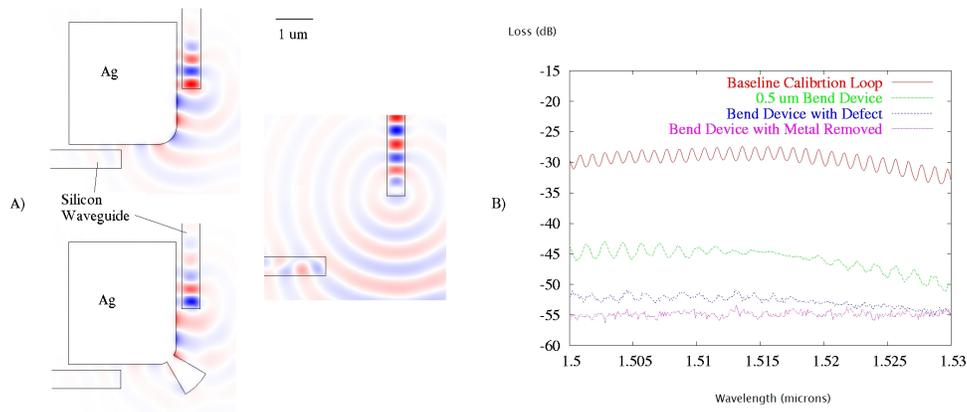
Fig. 4. Device layouts and renderings from FDTD simulations are shown in A), for the non-defective, metal-free, and defective devices, clockwise from top left. The out-of plane H field is rendered as blue and red. In B), the transmission spectra of the best measured devices of each type are shown, with fiber to fiber insertion loss in dB plotted against laser wavelength in  $\mu\text{m}$ . The baseline calibration loop spectrum is also shown for comparison.
