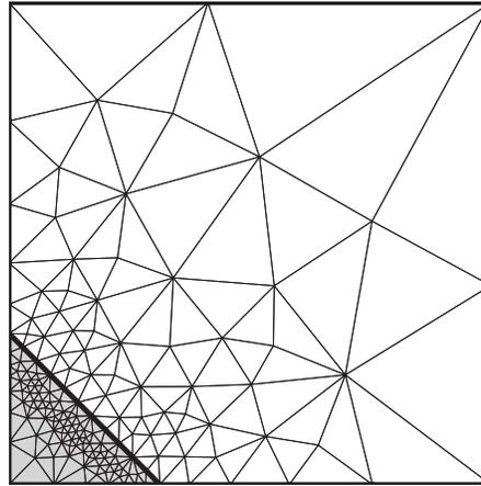
Figure 5.1: Initial inclusion shape and finite-element mesh adopted in the computation of the equilibrium shapes of inclusions.
