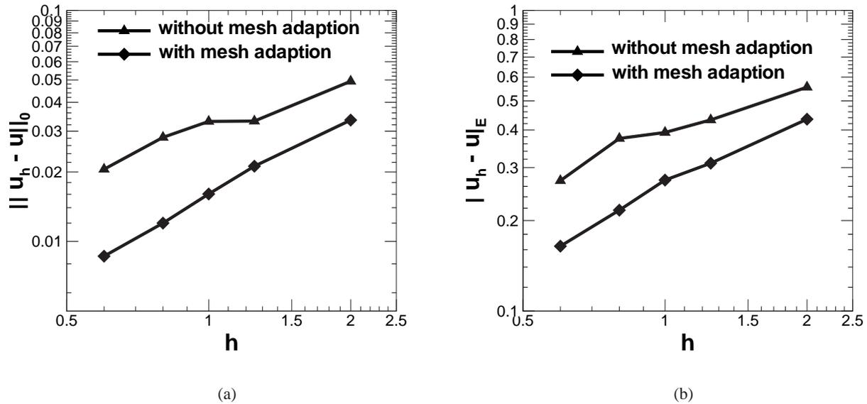
Figure 4.5: Three-dimensional analysis of a semi-infinite crack in a linear elastic solid subjected to mode I loading, convergence plots: a)  $L^2$ -norm of displacement error; b) Energy norm of displacement error.
