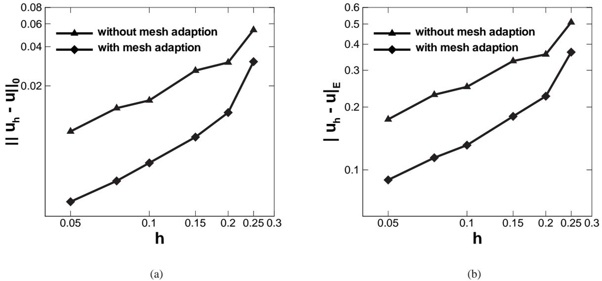
Figure 4.3: Two-dimensional analysis of a semi-infinite crack in a linear elastic solid subjected to mode I loading, convergence plots: a)  $L^2$ -norm of displacement error; b) Energy norm of displacement error.
