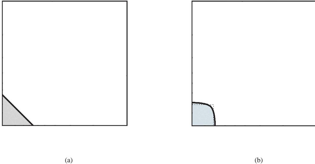
Figure 5.3: Equilibrium shapes a cubic inclusion/matrix system,  $C_{11} = 200$  GPa,  $C_{12} = 100$  GPa, and  $C_{44} = 150$  GPa,  $\epsilon^* = 0.01$ ,  $\gamma = 50$  mJ/m<sup>2</sup>. a) Initial shape of a 40 nm inclusion. b) Computed equilibrium shape of the inclusion.
