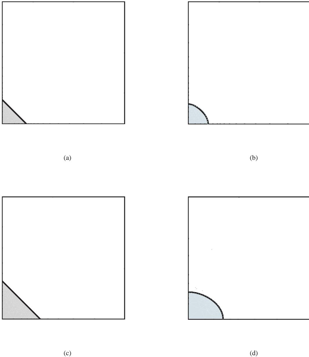
Figure 5.2: Equilibrium shapes an isotropic inclusion/matrix system,  $E^{\text{inc}} = 100$  GPa,  $E^{\text{mat}} = 150$  GPa,  $\nu = 1/3$ ,  $\epsilon^* = 0.01$ ,  $\gamma = 50$  mJ/m<sup>2</sup>, and  $r_c = 35.62$  nm. a) Initial shape of small ( $r = 31.91$  nm  $< r_c$ ) inclusion. b) Computed and analytical (red) equilibrium shape of small inclusion. c) Initial shape of large ( $r = 39.89$  nm  $> r_c$ ) inclusion. d) Computed and analytical (red) equilibrium shape of large inclusion.
