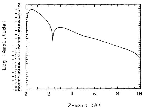
FIG. 3. Log plot of the absolute amplitude of the HOMO (donor orbital) in the  $\text{MoS}_2 \cdots \text{Ba}$  sample-tip system. The amplitude is calculated along a line perpendicular to the surface and passing through the central Mo and the Ba. The Mo plane is at  $z = 0$  Å, the S plane is at  $z = 1.49$  Å, and the Ba tip is at  $z = 10.0$  Å.
