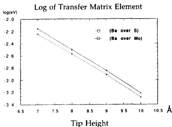
FIG. 4. Log plot of  $T_{BA}$  for the  $\text{MoS}_2$ -Ba sample-tip system as a function of tip atom distance over the Mo plane (at 0 Å). For the solid line, the tip was over the central cluster Mo. For the dashed lined, the tip was over a cluster S. The units of  $T_{BA}$  were eV.
