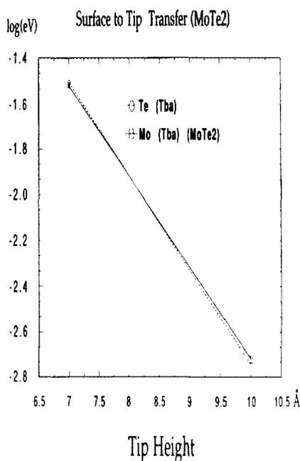
FIG. 5. Log plot of  $T_{BA}$  for the  $\text{MoTe}_2$ -Ba sample-tip system as a function of tip atom distance over the Mo plane (at 0 Å). For the solid line, the tip was over the central cluster Mo. For the dashed lined, the tip was over a cluster Te. The units of  $T_{BA}$  were eV.
