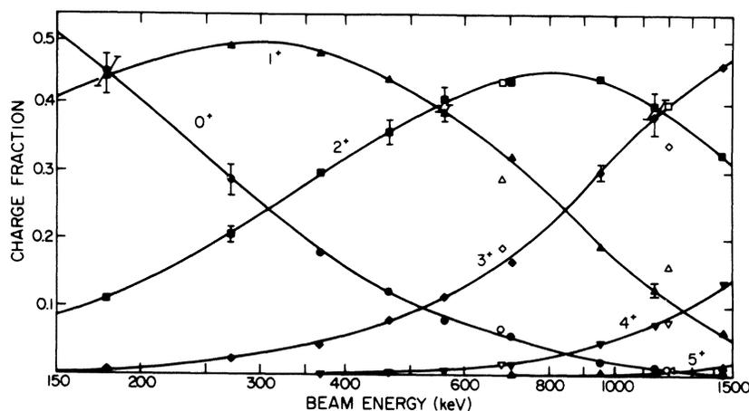
FIG. 3. Equilibrium charge distribution for nitrogen in carbon foils. The open symbols refer to data from Ref. 7. Root-mean-square deviations less than  $\pm 0.02$  are not shown. The curves are drawn to aid the eye.
