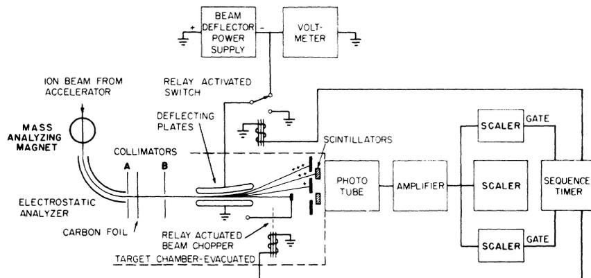
FIG. 1. Schematic diagram of charge-distribution measurement apparatus.
