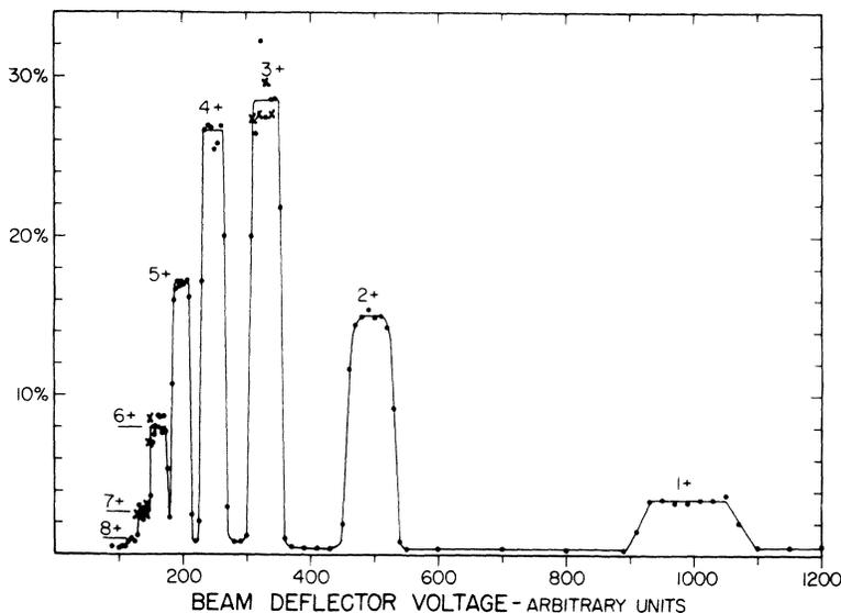
FIG. 2. Ratio of counts in upper scintillator to counts in lower scintillator as a function of the voltage on the deflector plates for argon at 1450-keV beam energy. The circles and crosses refer to separate sets of measurements. The curve is drawn to aid the eye.
