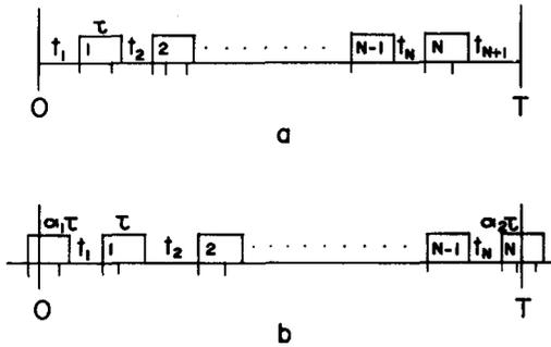
FIG. 1. Tick marks below the line represent actual events. Rectangles above the line, which represent system dead times of length  $\tau$ , occur after each recorded count. Intervening live times are labeled by  $t_1, t_2, \dots$ , and  $\alpha_1, \alpha_2$  denote fractions of dead times occurring inside the counting interval. In general,  $0 \leq \alpha_1, \alpha_2 \leq 1$ . (a) Ideal case; (b) less ideal case.
