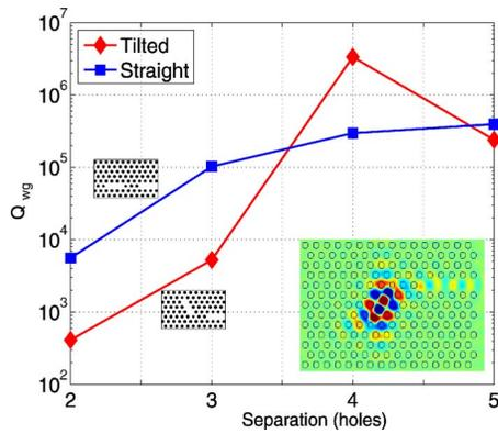
FIG. 2. (Color online) Simulation results for the cavity-waveguide coupling expressed in terms of the quality factor. The coupling strength is proportional to  $(1/Q_{wg})$ . Simulated magnetic field of a cavity-waveguide coupler in tilted configuration with three-hole separation (inset).
