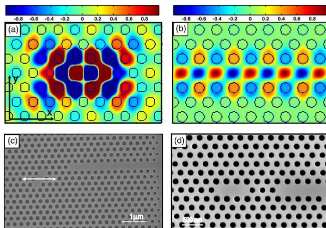
FIG. 1. (Color online) (a) Magnetic field ( $B_z$  component) for the mode with the highest quality factor in a L3 cavity. (b) Magnetic field pattern of the even mode in a PC waveguide. (c) Fabricated tilted cavity coupled to a waveguide (four-hole separation). In this experiment we shift the cavity with respect to the waveguide along the direction indicated by the arrow. (d) Fabricated straight cavity coupled to a waveguide (three-hole separation).
