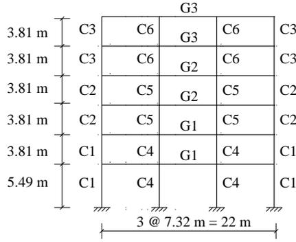
**FIG. 3. Moment-resisting frame structure**
