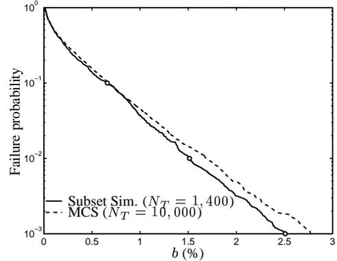
**FIG. 5. Failure probability estimates for Case 2**
