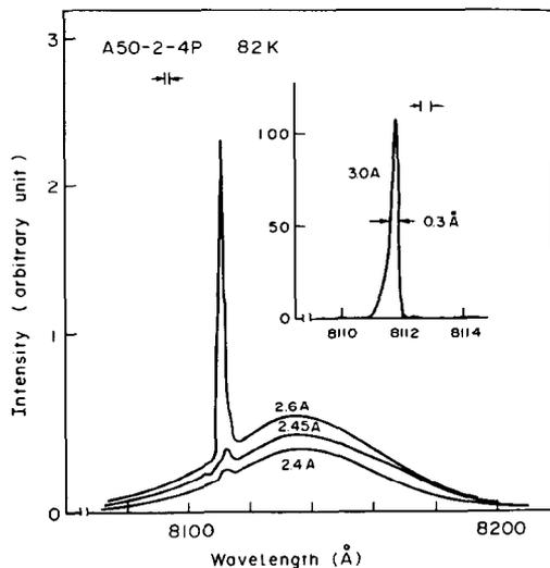
FIG. 8. The emission spectra of a typical laser. The period and the depth of the corrugation is 3470 and 1800 Å, respectively. The threshold current density is 750 A/cm<sup>2</sup> at 80° K.
