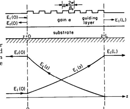
FIG. 2. The behavior of the incident and reflected wave in a periodic waveguide with gain.
