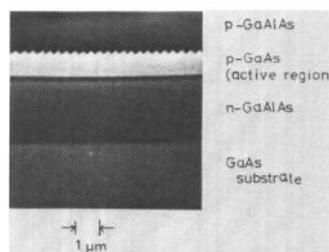
FIG. 6. A SEM photograph of the cross section of a distributed-feedback laser along the direction of light propagation. The corrugation period is  $3470 \text{ \AA}$ .
