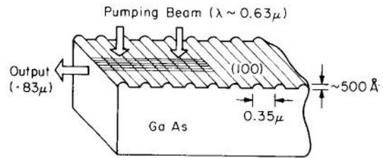
FIG. 5. Schematic structure of a GaAs distributed-feedback laser.
