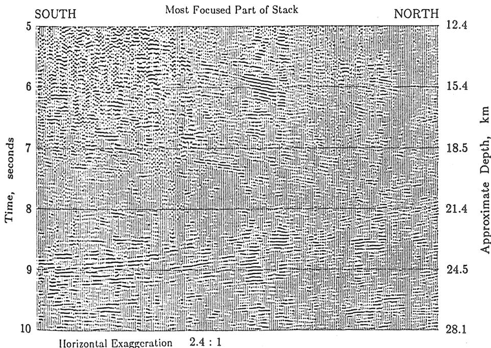
Figure 4. Stack of deep reflections from the CALCRUST Ward Valley wide-angle survey showing the true amplitude of the reflections multiplied by the semblance focusing of the stack, over 8.3 km of midpoints. The strongest reflections are from the top of the basal-crustal zone at 8.4 s and from the Moho at 9.5 s.
