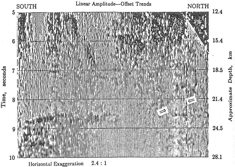
**Figure 5.** Image of the linear reflection amplitude dependence on offset for each point of the stack of Fig. 4. Dark areas indicate an increase in amplitude with offset. Most of the strong reflections result from classical discontinuities, but the south-dipping reflection on the lower right (between arrows) may be from a strong contrast in anisotropy, or an inclusion of pore fluid.
