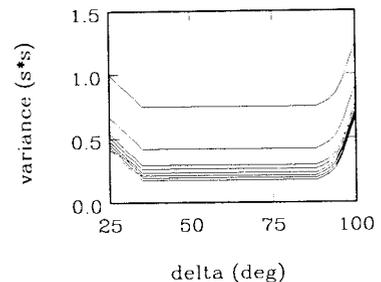
**Figure 6.** The variation of random-error variance with epicentral distance and source depth for the  $P$ -wave data. The different curves represent different source depths, with the highest variance for shallow events, and the variance monotonically decreasing with source depth. The eight curves are 100 km increments in depth.
