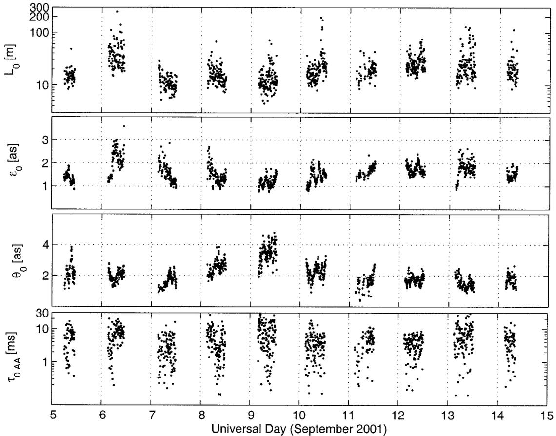
Fig. 1. Atmospheric parameters measured by the GSM at the Palomar Observatory:  $L_0$  is the outer scale of turbulence,  $\epsilon_0$  is the seeing FWHM (as inferred from atmospheric coherence diameter  $r_0$ ),  $\theta_0$  is the isoplanatic angle, and  $\tau_{0AA}$  is the angle-of-arrival atmospheric coherence time.
