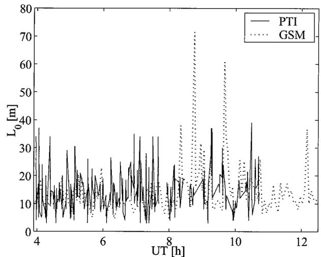
Fig. 6. Typical results for outer-scale of turbulence  $L_0$  as measured by the GSM and by the PTI interferometer. We deduced the  $L_0$  values obtained with the PTI by fitting the measured fringe speed with the theoretical expression given in Subsection 2.C. These data were obtained during the night of 9 September 2001 at the Palomar Observatory.
