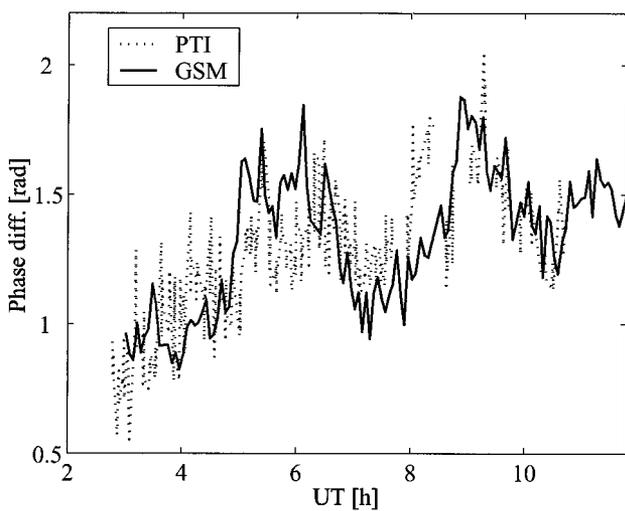
Fig. 5. Typical results for temporal differential variance (fringe speed multiplied by sampling time) measured with the PTI interferometer and modeled from the GSM data. These data were obtained during the night of 9 September 2001 at the Palomar Observatory.
