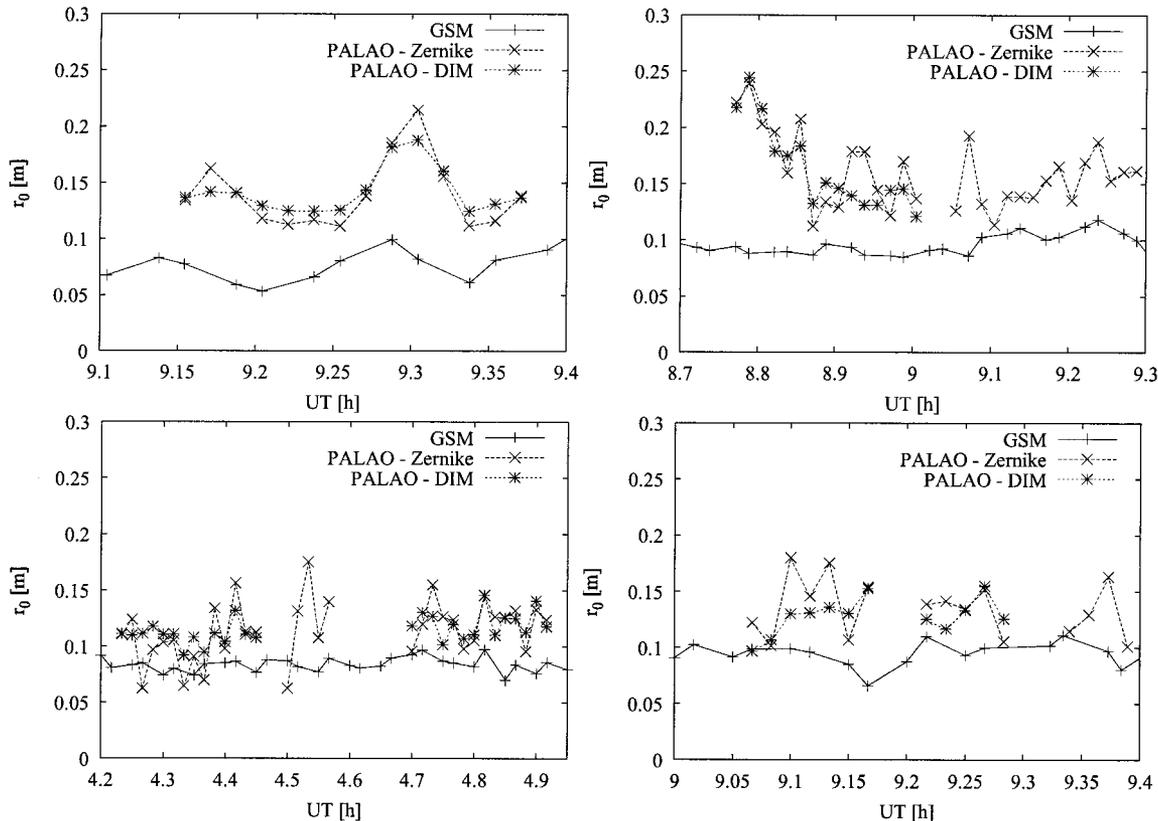
Fig. 3. Comparison of atmospheric coherence length  $r_0$  measurements obtained with the GSM and from PALAO telemetry data during the nights of 7, 8, and 9 September 2001 (respectively, top left, top right, and bottom) at the Palomar Observatory. Differences are due to the different locations of the instruments and display the expected behavior, as explained in the text.
