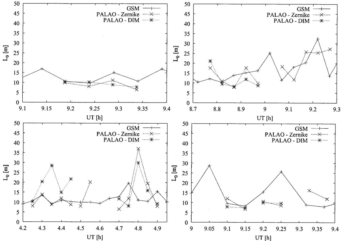
Fig. 4. Comparison of outer-scale of turbulence ( $L_0$ ) measurements obtained with the GSM and from PALAO telemetry data during the nights of 7, 8, and 9 September 2001 (respectively, top left, top right, and bottom) at the Palomar Observatory. These results are to our knowledge the first independent verification of the validity of our method to determine  $L_0$  from AO telemetry data.
