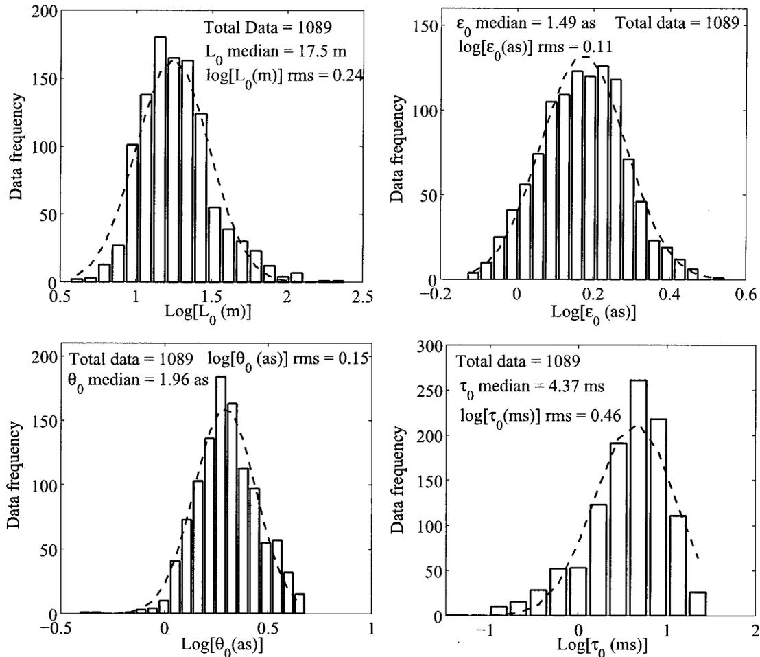
Fig. 2. Distributions of the atmospheric optical parameters obtained with the GSM at the Palomar Observatory in September 2001. Dashed curves, best-fit log-normal distributions.
