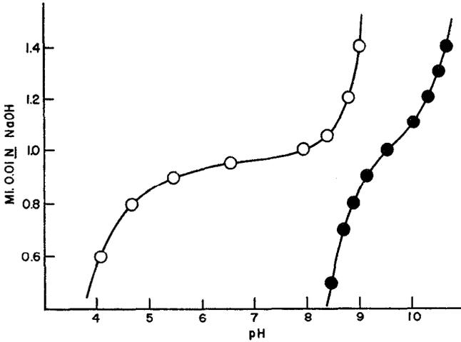
FIG. 1. Titration of tris(hydroxymethyl)aminomethane-hydrochloric acid buffer. ●, 2.0 ml. of 0.01 M buffer; ○, 1.0 ml. of 0.02 M buffer and 1.0 ml. of 36 per cent aqueous formaldehyde adjusted to pH 7.0.
