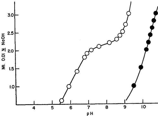
FIG. 2. Titration of ethylenediamine-hydrochloric acid buffer. ●, 2.0 ml. of 0.01 M buffer; ○, 1.0 ml. of 0.02 M buffer and 1.0 ml. of 36 per cent aqueous formaldehyde adjusted to pH 7.0.
