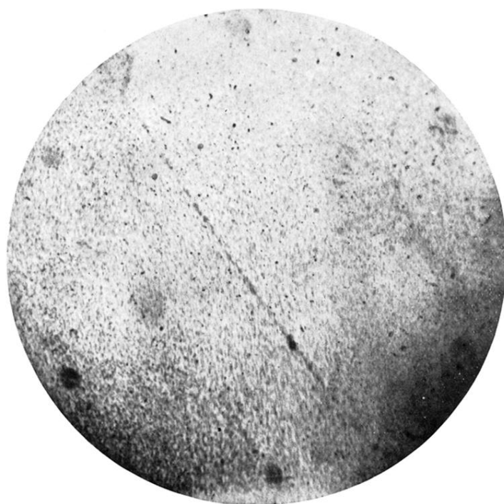
Fig. 16. 12,000 gauss. A proton of 30 \times 10^6 volts energy.
