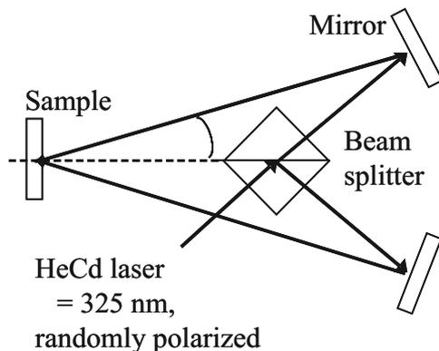
Fig. 1. Setup used for holographic recording.
