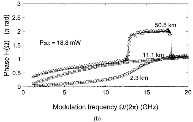
Fig. 5. Measured change in modulation response after 2.3 km (circles), 11.1 km (squares) and 50.5 km (triangles) of standard fiber together with theoretical curve using frequency dependent  $\kappa(\Omega)$ . Output power at laser facet = 18.8 mW.
