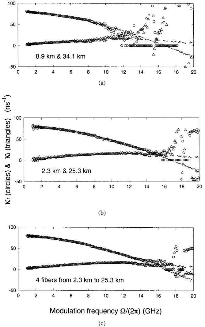
Fig. 3. Real (circles) and imaginary (triangles) part of  $\kappa(\Omega)$  with  $\alpha = -5.5$  obtained from  $|H(\Omega, z)|^2$  for different combinations of fiber. Solid and dashed curves are the result from using magnitude and phase of  $H(\Omega, z)$ . Output power at laser facet = 18.8 mW.
