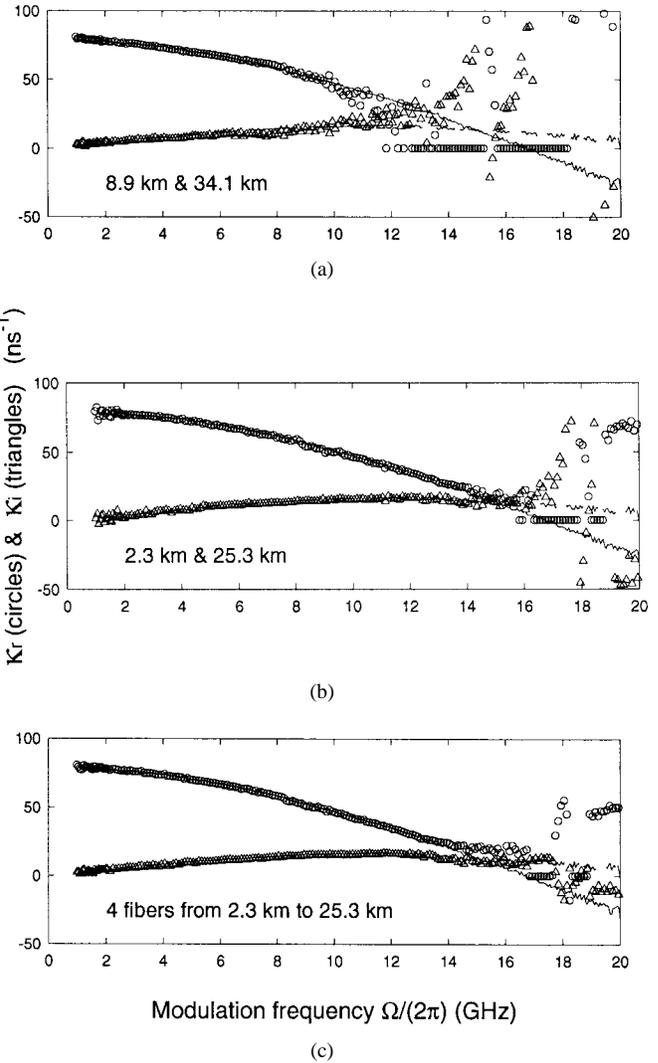
Fig. 3. Real (circles) and imaginary (triangles) part of  $\kappa(\Omega)$  with  $\alpha = -5.5$  obtained from  $|H(\Omega, z)|^2$  for different combinations of fiber. Solid and dashed curves are the result from using magnitude and phase of  $H(\Omega, z)$ . Output power at laser facet = 18.8 mW.
