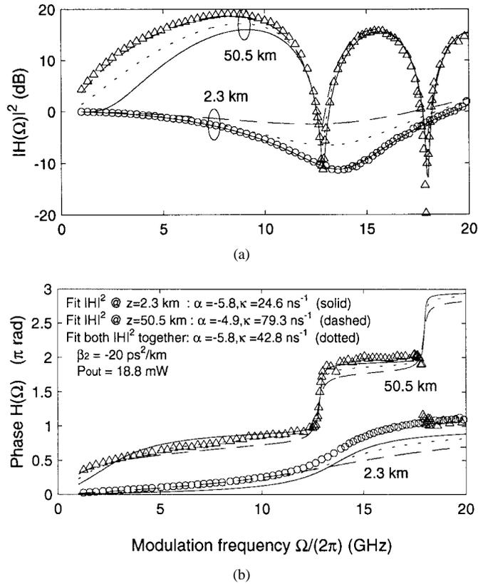
Fig. 2. Change in modulation response after 2.3 km (circles) and 50.5 km (triangles) of standard fiber at 1.54  $\mu$ m. The parameters  $\kappa$  and  $\alpha$  are determined that best fit the change in modulation response after 2.3 km (solid), 50.5 km (dashed), and both lengths of fiber (dotted). Output power at laser facet = 18.8 mW.
