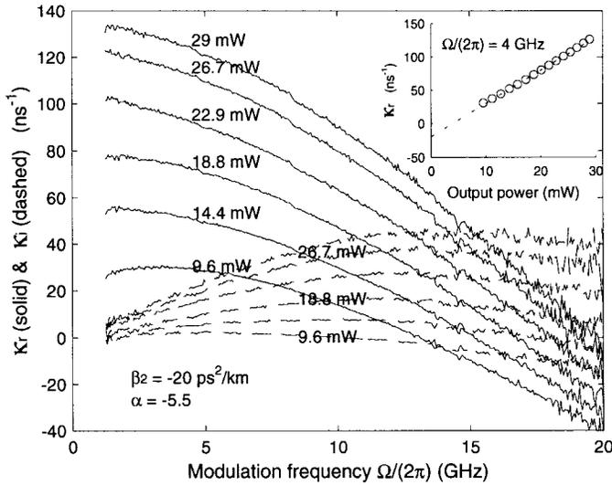
Fig. 4. Real (solid) and imaginary (dashed) part of  $\kappa(\Omega)$  with  $\alpha = -5.5$  at several laser output powers from magnitude and phase of  $H(\Omega, z)$ . The inset shows the real part of  $\kappa(\Omega)$  as a function laser output power (circles) together with a linear fit (dotted) at  $\Omega/2\pi = 4$  GHz.
