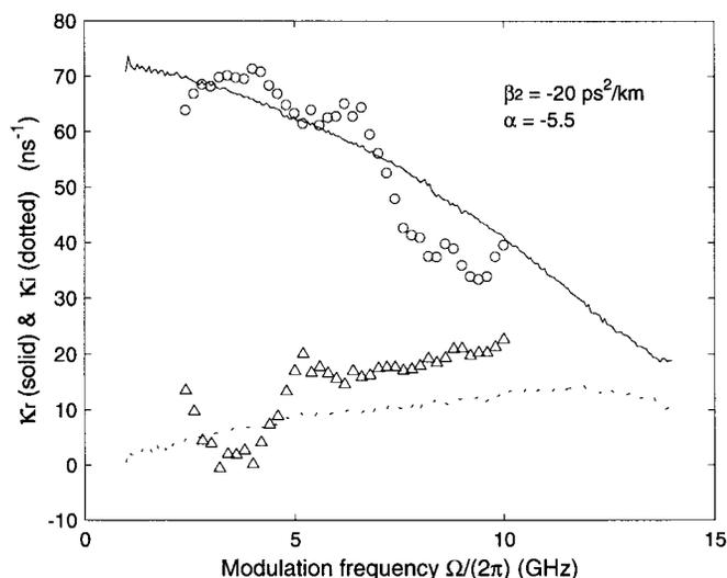
Fig. 7. Real and imaginary part of  $\kappa(\Omega)$  obtained from modulation response (solid and dashed, respectively) and from optical spectrum side bands (circles and triangles, respectively). Output power at laser facet = 16.3 mW.
