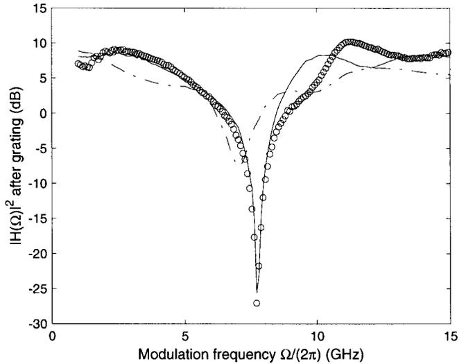
Fig. 6. Baseband transfer function after transmission through fiber grating predicted using frequency dependent  $\kappa(\Omega)$  (solid) and constant  $\kappa$  (dashed) compared to measurement (circles).
