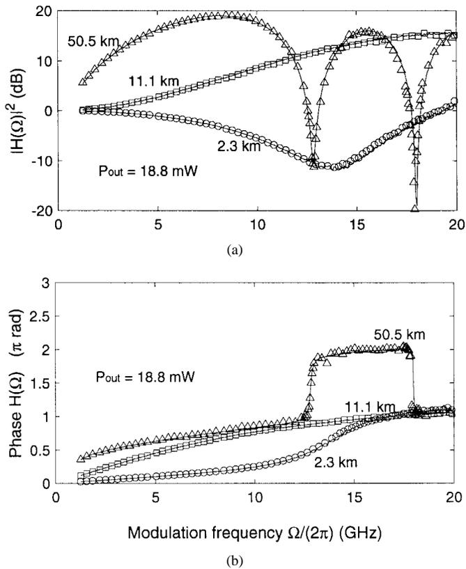
Fig. 5. Measured change in modulation response after 2.3 km (circles), 11.1 km (squares) and 50.5 km (triangles) of standard fiber together with theoretical curve using frequency dependent  $\kappa(\Omega)$ . Output power at laser facet = 18.8 mW.
