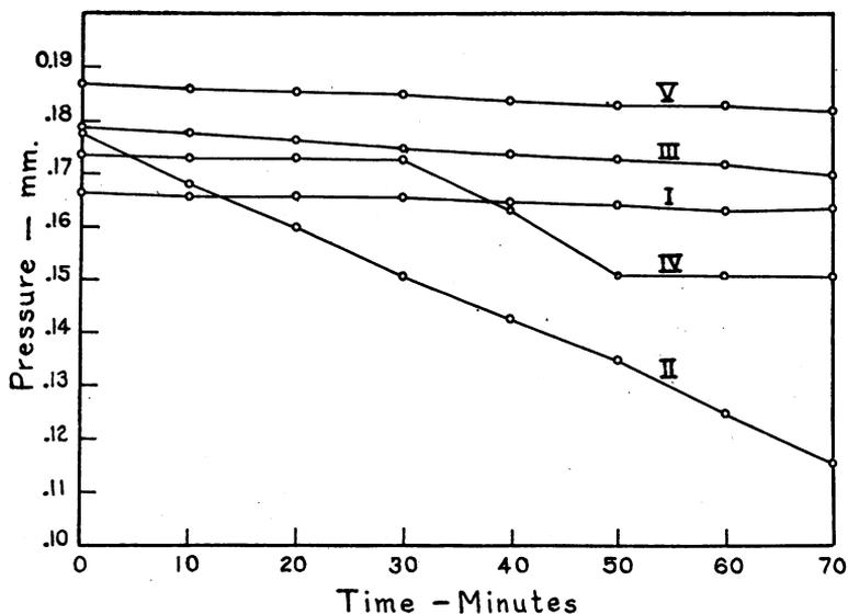
differed from II only in having no air blast in the first 30 and last 20 minutes. V differed from II only in having no mercury present in the reaction tube. The rate of decrease of pressure in experiments like V seemed to depend greatly on the care used to remove all traces of mercury from the reaction tube; in some trials almost no decrease was observed.
