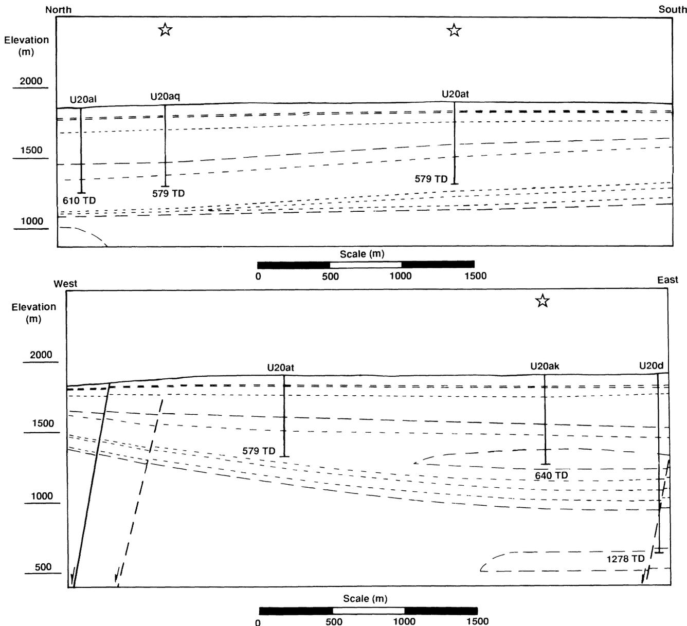
FIG. 1. The geologic strata in area 20 of the Nevada Test Site are typically a series of horizontal lava flows interspersed with alluvial material. Borehole U20AK is at the center of a cluster of five holes that we have studied. North-South and East-West cross sections through this area are shown, adopted from Ref. 7.
