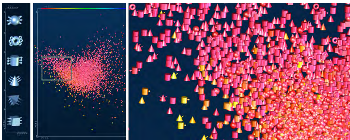
Fig. 1. (Left) Six unique 3D glyphs used to map the angle between two particle tracks ( d\phi_1 ) from a high energy physics detector simulation. Left “arm” features on glyph map energy from one photon ( eg_1 ), right “arms map energy from second photon ( eg_2 ). (middle) Scatterplot mapping two principal components to (x,y) position. Glyph hue represents Higgs Mass. (Right) Close up of left branch of scatterplot. Lower-right Dense plot area is easily recognizable as mostly spheres (low angle) but for few tori and cylinders. Upper-left area shows mostly cylinders and cones. Few objects show high energy as expected to correlate to mass.
