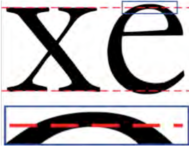
Fig. 3. Classic example of typographic design, where curved shapes (letters) are drawn beyond the guide lines ( base line and x-height overhang) to allow letters to seem visually equivalent in height. Shown font is Adobe's Garamond.
