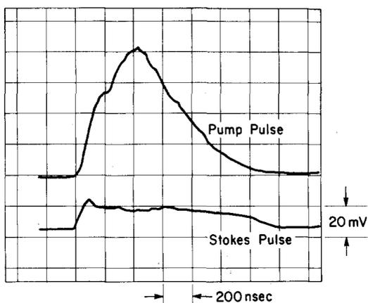
FIG. 3. Oscilloscope traces of pump pulse and spin-flip output pulse. Both were taken with the same amplifier gain setting.
