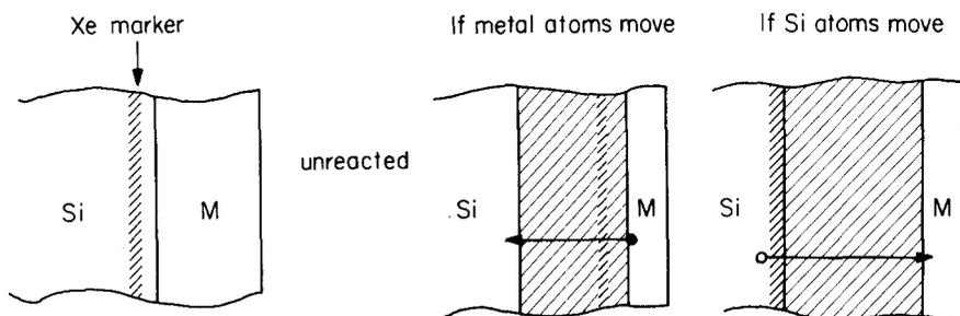
FIG. 1. Schematic diagrams of implanted marker and marker displacements during silicide formation. The marker will shift toward the surface if metal atoms are the dominant diffusion species and will shift deeper into the sample if the dominant diffusing species is silicon.
