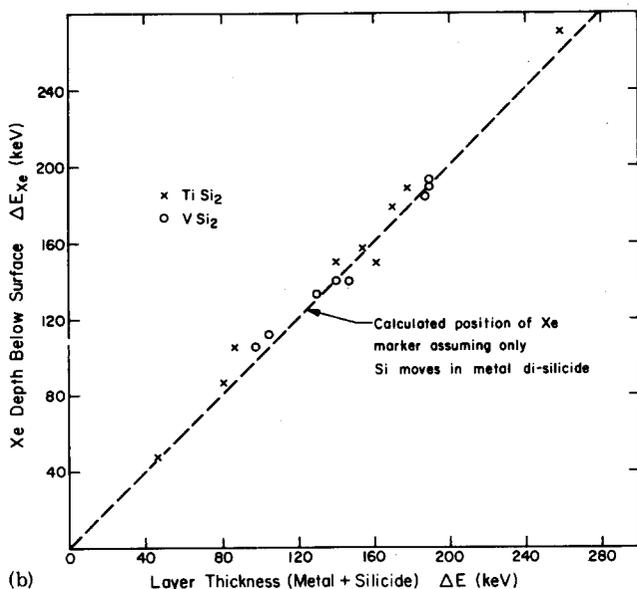
FIG. 3. (a) The sketched energy spectra of backscattered ions from a V/Si sample before and after the  $VSi_2$  formation. The displacement into the Si of the implanted Xe markers can be seen at the high-energy side. (b) The amount of displacement of the Xe marker vs the thickness of the metal plus silicide layer. The dashed line corresponds to the energy shift of the Xe under the assumption that Si is the diffusing species.
