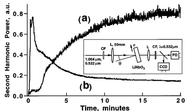
FIG. 1. Growth of SH with time (a) for  $16^\circ$  angle of incidence, (b) for normal incidence. Optical power at  $1.064 \mu\text{m}$  is 1.5 W. Inset: experimental setup. L is a lens, PD is a photodetector, CF's are appropriate color filters.
