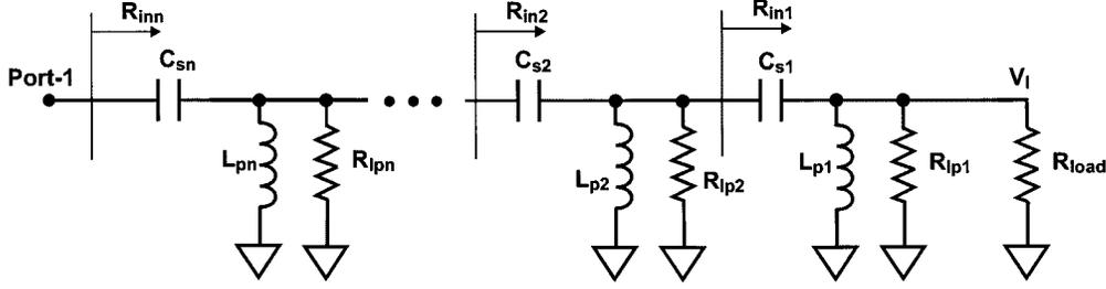
Fig. 5. Multisection resonant LC impedance-transformation network with loss.
