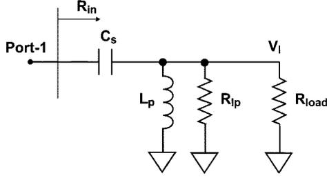
Fig. 2. Resonant LC impedance-transformation network with loss.
