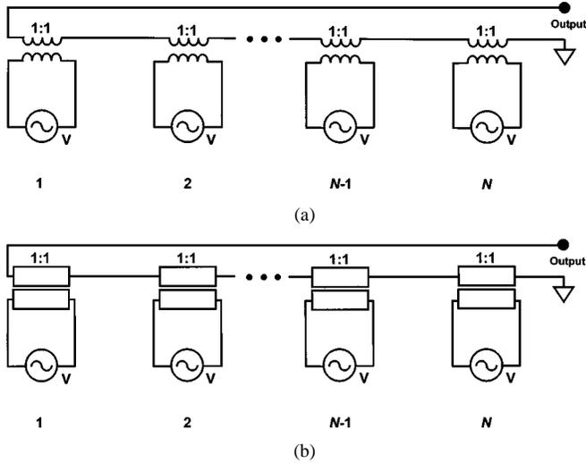
Fig. 13. (a) Fundamental building block of DAT.  $N$  independent power sources combined in series through  $N$  transformers with turn ratio 1:1. (b) Same diagram using coupled slab inductors as the transformer.
