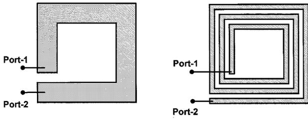
Fig. 19. One-turn planar spiral inductor and multturn planar spiral inductor.
