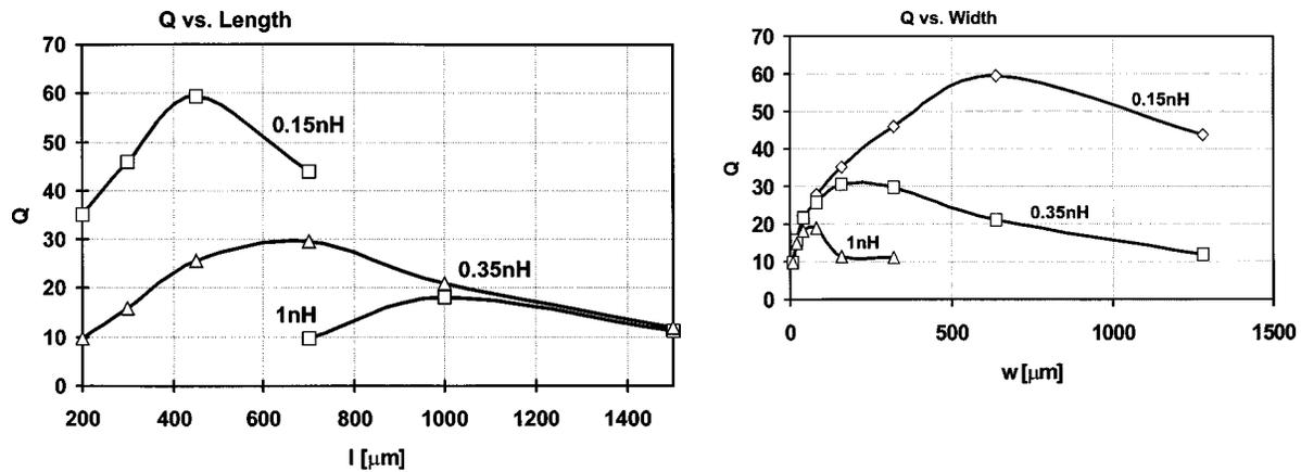
Fig. 23.  $Q$  of a transmission-line inductor versus metal length or metal width and inductance. In the first plot, for each metal length, the width, which provides the selected inductance, is chosen. In the second plot, for each metal width, the length, which provides the selected inductance, is chosen.
