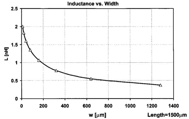
Fig. 21. Inductance of a transmission-line inductor versus metal width for constant metal length (1500  $\mu\text{m}$ ).
