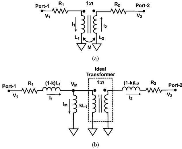
Fig. 7. (a) Transformer model. (b) Transformer equivalent T-model.
