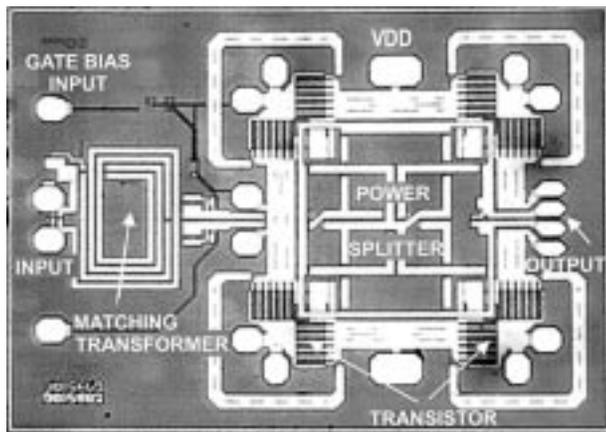
Fig. 18. Microphotograph of the measured DAT power amplifier.
