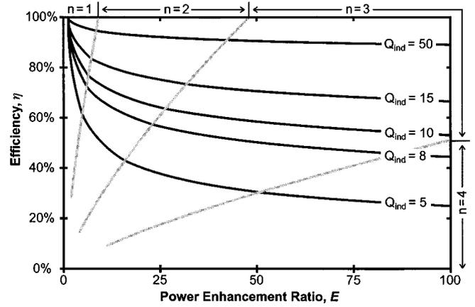
Fig. 6. Efficiency versus PER and inductor  $Q$  for a multisection resonant network. Vertical gray lines separate regions using different number of sections. The best number of sections  $n$  from 1–4 is chosen for the highest efficiency for different PERs and inductor  $Q$ .
