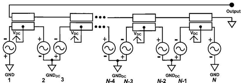
Fig. 14.  $N$  independent power sources combined in series through  $N/2$  transformers in double-differential configuration with grounds shared between adjacent power sources, except for the first and last sources in the chain.
