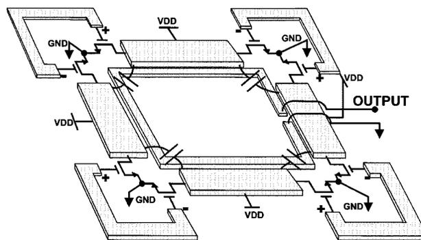
Fig. 16. Representative drawing of a complete DAT with 8 NMOS transistors.
