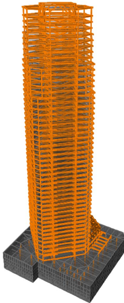
Figure 9. Finite-element ETABS model of 52-story building based on information about structural and connection elements obtained from structural engineering drawings.
