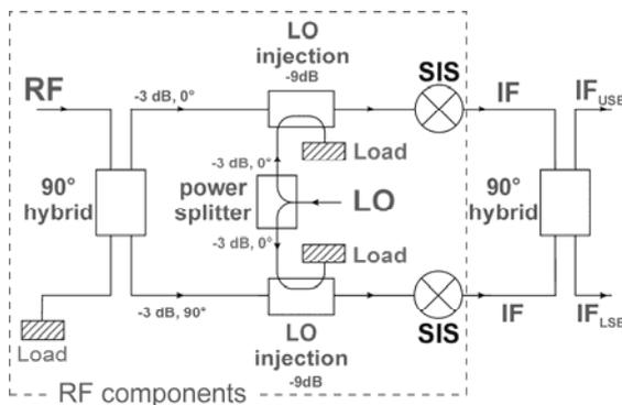
**Figure 1.** Schematics of the selected 2SB configuration. The incoming RF signal is divided in a  $90^\circ$  hybrid. The split signals are combined with an LO signal and then mixed into two SIS junctions. The resulting down converted signals are fed into a second hybrid after which the IF signals corresponding to the lower and upper sideband are obtained in two different channels.
