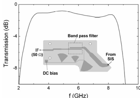
**Figure 6.** Calculated transmission between the input and output ports of the IF structure presented in the inset.
