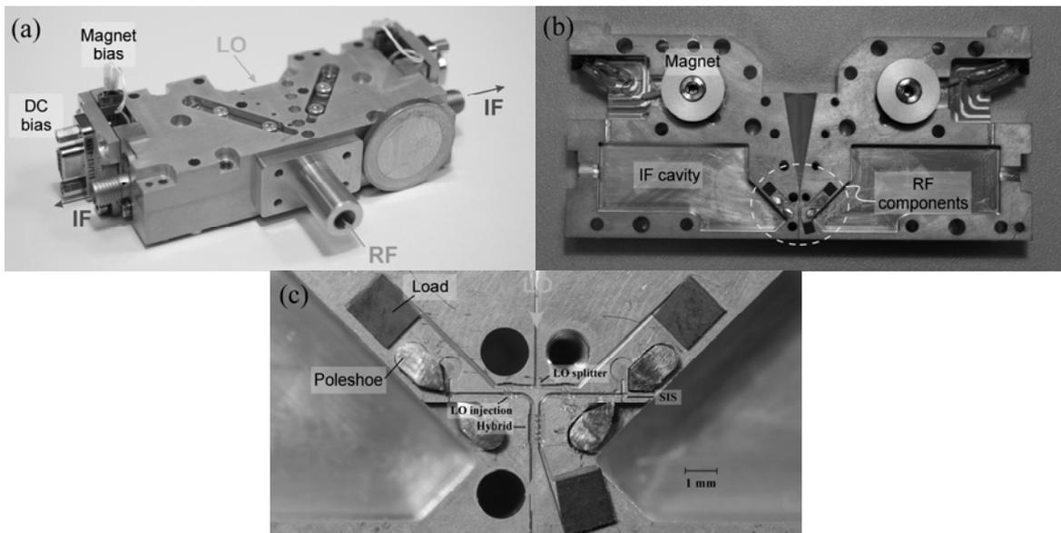
**Figure 7.** (a) Constructed 2SB block. (b) Upper half. (c) Close-up of the RF components.
