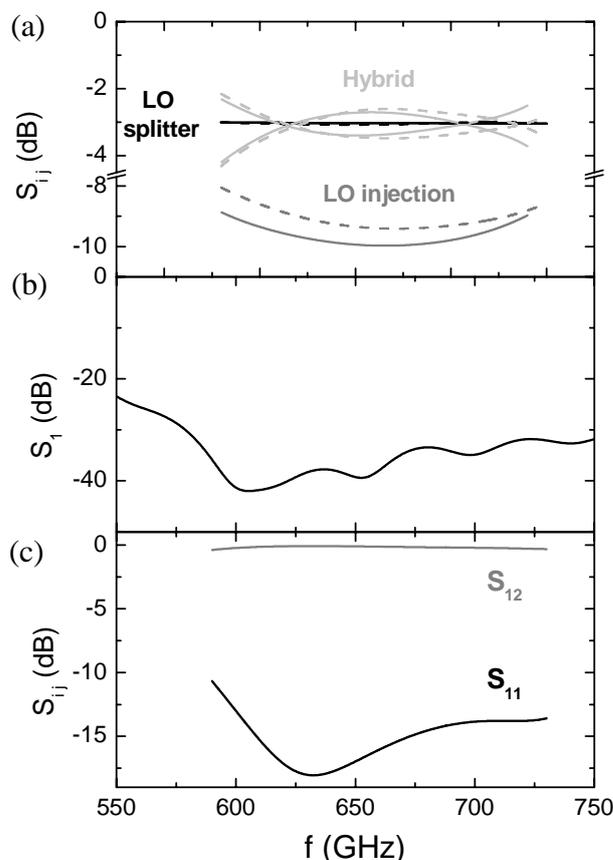
**Figure 3.** Results of the electromagnetic simulation of the different RF components: (a) S-parameters between the input and output of the the 90° hybrid, LO splitter, and LO injector as designed, solid lines, and as constructed, dashed lines. (b) Reflection coefficient of the signal termination load. (c) Coupling efficiency and return loss of the waveguide-microstrip transition.
