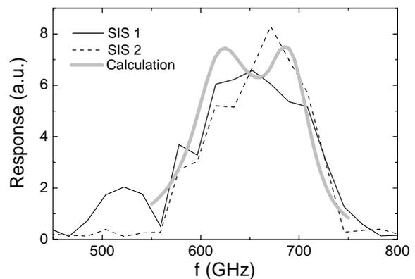
**Figure 5.** Calculated and measured response of the fabricated SIS junctions. The response was measured through the RF port.
