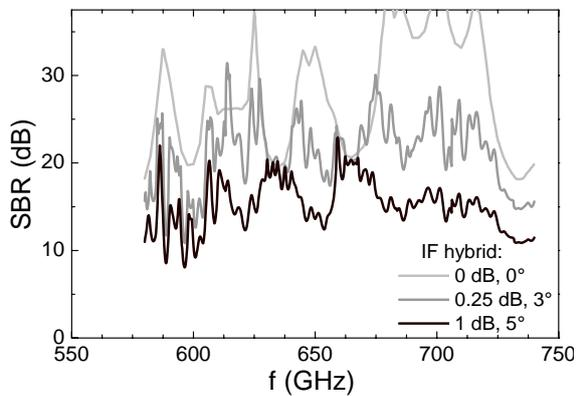
**Figure 4.** Calculated SBR assuming a perfect IF hybrid (light gray) and with a amplitude and phase imbalances of 0.25 dB and 3° (gray), and 1 dB and 5° (black).
