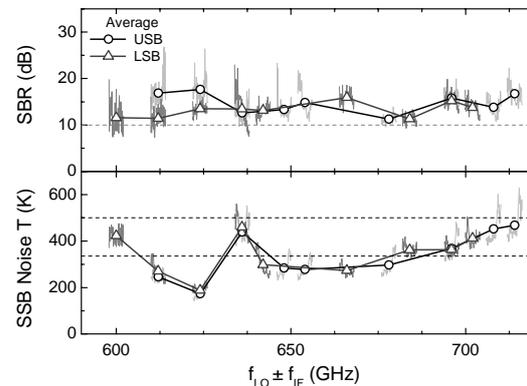
**Figure 9.** Single sideband noise temperatures (bottom panel) and image rejection ratios (upper panel) at different LO frequencies. Both parameters are close to ALMA specifications (horizontal dashed lines) described in the text.
