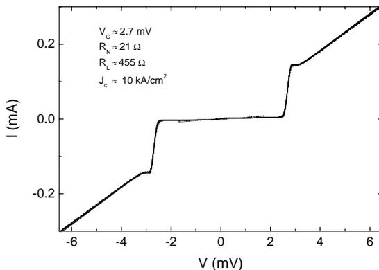
**Figure 8.** IV curves of 8 different junctions. The average values of gap voltage ( $V_G$ ), normal resistance ( $R_N$ ), leakage resistance ( $R_L$ ), and critical current density ( $J_C$ ) are shown.
