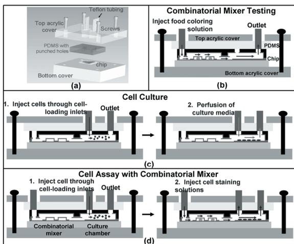
Fig. 3 (a) Schematic representation of the packaging method. Chip packaging for various device operations: (b) combinatorial mixer testing, (c) cell culturing experiment, (d) cell assay with combinatorial mixer.
