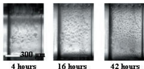
Fig. 6 Cell culture on chip. B35 cells attached to the surface 4 hours after cell loading and proliferated. Pictures were taken 4 hours, 16 hours and 42 hours after cell loading.
