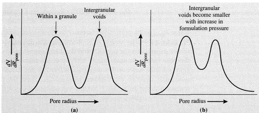
**Figure 6.3.2** | Influence of pelletizing conditions on pore size distribution  $\frac{dV}{dR_{\text{pore}}}$  in a bimodal pore network. **(a)** Small pores (micropores) are associated with the catalyst powder whereas large pores (macropores) result from the voids between granules in compressed catalyst pellets. **(b)** Decrease in pore size associated with intergranular voids as pellet in **(a)** is compressed as higher pressure.
