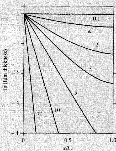
**Figure 6.4.4** | Growth rate profiles in the macrocavity reactor predicted by Equation 6.4.39. Film thickness is normalized by the value at inlet of the cavity. (Adapted from K. Watanabe and H. Komiyama, "Micro/Macrocavity Method Applied to the Study of the Step Coverage Formation Mechanism of SiO<sub>2</sub> Films by LPCVD," *J. Electrochem. Soc.*, 137 (1990) 1222, with permission of the Electrochemical Society, Inc.)
