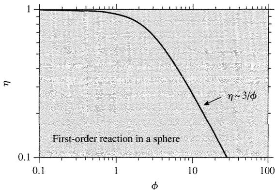
**Figure 6.3.8 |** Effectiveness factor for a first-order reaction in a sphere as a function of the Thiele modulus.
