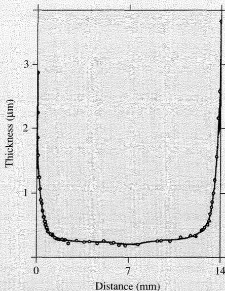
**Figure 6.4.3** | Growth rate profile of  $\text{SiO}_2$  in the macrocavity. (Reproduced from K. Watanabe and H. Komiyama, "Micro/Macrocavity Method Applied to the Study of the Step Coverage Formation Mechanism of  $\text{SiO}_2$  Films by LPCVD," *J. Electrochem. Soc.*, **137** (1990) 1222, with permission of the Electrochemical Society, Inc.)
