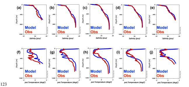
**Supplementary Figure 9.** Observed and simulated vertical profiles of potential temperature and salinity at the locations indicated by the black triangles along section C in Supplementary Figure 8 (ordered from left to right).
