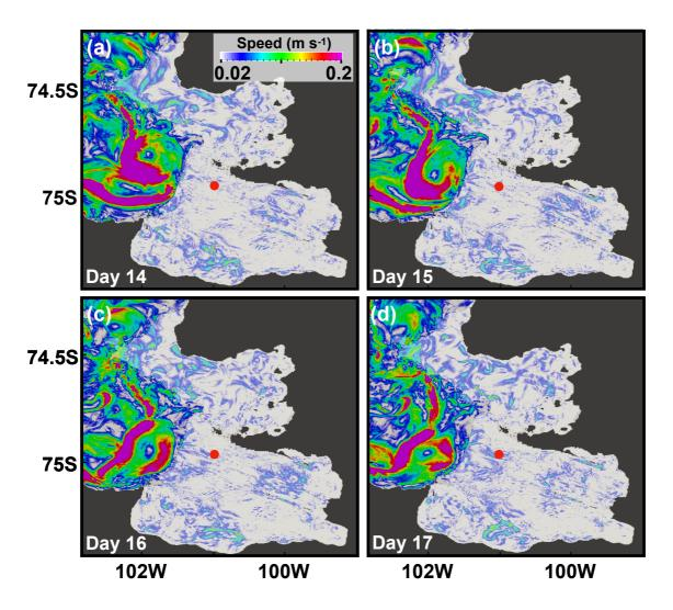
**Supplementary Figure 21.** Ocean speed anomaly 50 m below ocean top cells (below ice shelf for the cavity environment) for days (a) 14, (b) 15, (c) 16, and (d) 17. Ice shelves are shown with partially-transparent white patches, similar to Figure 1.
