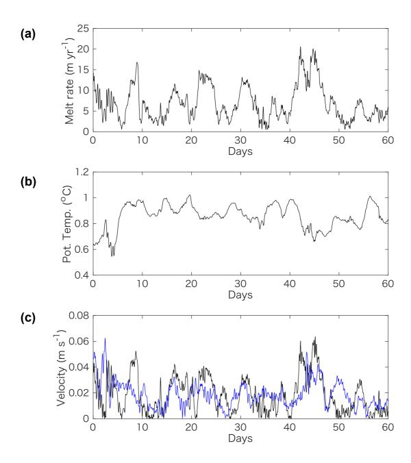
**Supplementary Figure 20.** (a) Time series of (a) simulated PIIS melt rate at the location of ApRES measurements for CTRL. Time series of simulated (b) potential temperature and (c) ocean speed below the ice shelf at the same location. Ocean speed 50 m below the uppermost model grid (blue) is also shown in (c).
