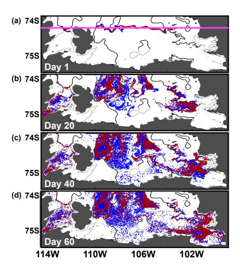
**Supplementary Figure 15.** Spatial distributions of particles initially released along 74.24° S (pink) after (a) 1, (b) 20, (c) 40, and (d) 60 days of model simulation. Red particles change their location based on hourly velocity fields, while blue particles change their location based on the 60-day mean model velocity field. For all panels, bathymetric contours of 500 m are shown (black).
