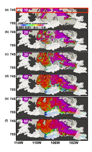
**Supplementary Figure 13.** (a) Spatial distributions of tracers representing CDW after (a) 10, (b) 20, (c) 30, (d) 40, (e) 50, and (f) 60 days of model simulation. The concentration of CDW tracer is set to 1.0 in the region north of 74.24° S (shown by the red box in (a)) and potential temperature higher than 1 °C. For all panels, bathymetric contours of 500 m are shown (black) and ice shelves are shown with partially-transparent white patches, similar to Figure 1.
