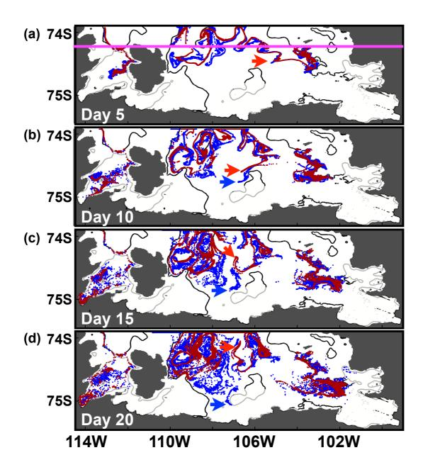
**Supplementary Figure 16.** Same as Fig. S8 but after (a) 5, (b) 10, (c) 15, and (d) 20 days of model simulation. Red and blue arrows are inserted to emphasize the difference of pathways for red and blue particles. After day 20, blue particles (indicated by blue arrow) travel towards the Thwaites ice shelf (TIS) grounding line.
