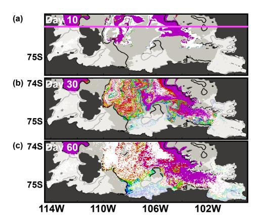
**Supplementary Figure 14.** Spatial distributions of particles (white points) initially released along 74.24° S (pink) after (a) 10, (b) 30, and (c) 60 days of model simulation. Horizontal distributions of CDW tracer (same as Fig. S6) are also shown to indicate that particles and CDW tracer behave similarly. For all panels, bathymetric contours of 500 m are shown (black) and ice shelves are shown with partially-transparent white patches, similar to Figure 1.
