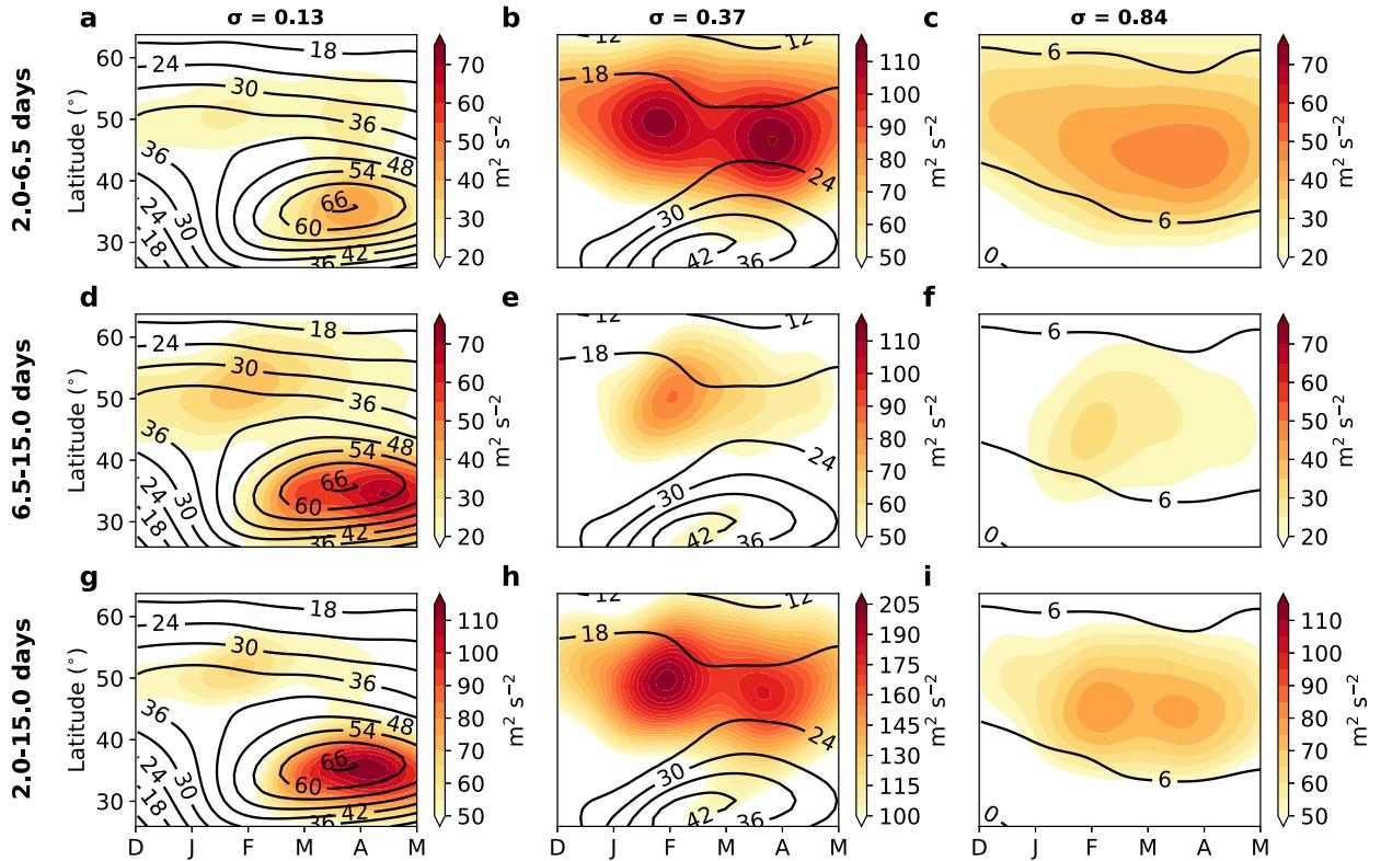
FIG. 4. Vertical dependency of the seasonal variability of meridional velocity variance  $\overline{v'^2}$  from the control run (oc10qf40) in the (left) lower stratosphere ( $\sigma = 0.13$ ), (center) upper troposphere ( $\sigma = 0.37$ ), and (right) lower troposphere ( $\sigma = 0.84$ ). Eddies are determined with bandpass filters with time scales of (a)–(c) 2–6.5, (d)–(f) 6.5–15, and (g)–(i) 2–15 days. Black contours are the zonal-mean zonal wind at that level.
