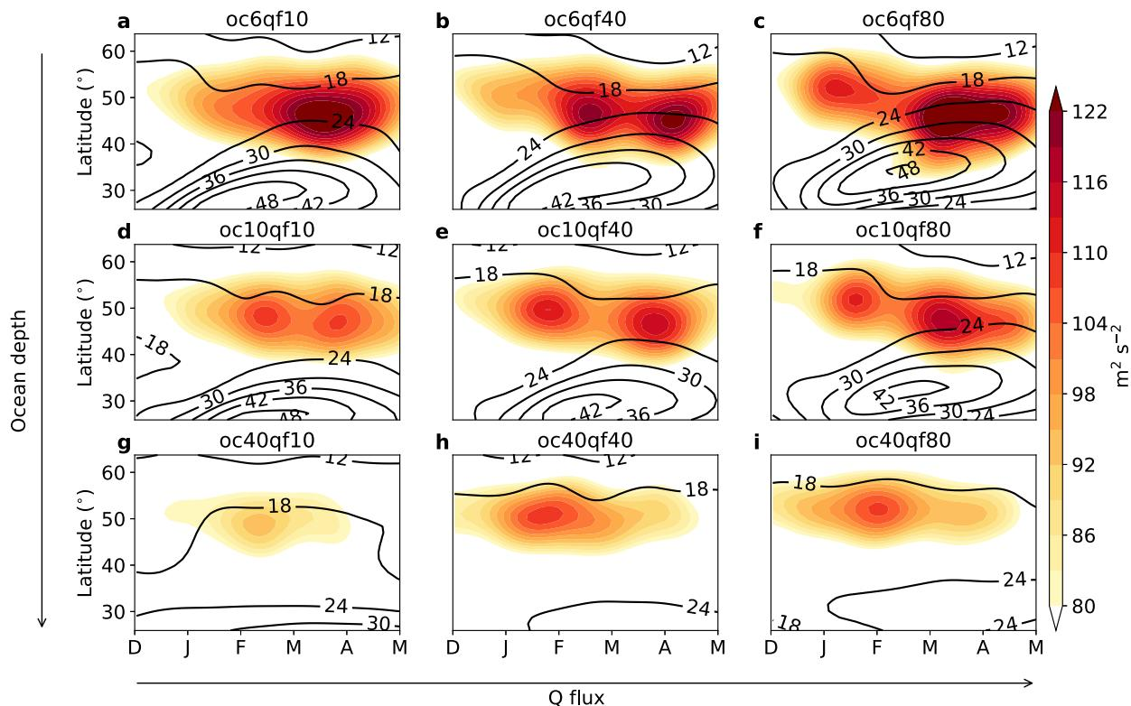
FIG. 6. Sensitivity in the GCM runs of the seasonal variability of  $\overline{v^2}$  (colors; at  $\sigma = 0.37$ ) and zonal wind (black contours; at  $\sigma = 0.37$ ) to changing  $Q$  fluxes and ocean depth. Eddies were computed using filter time scales of 2–6.5 days. (e) The control run.
