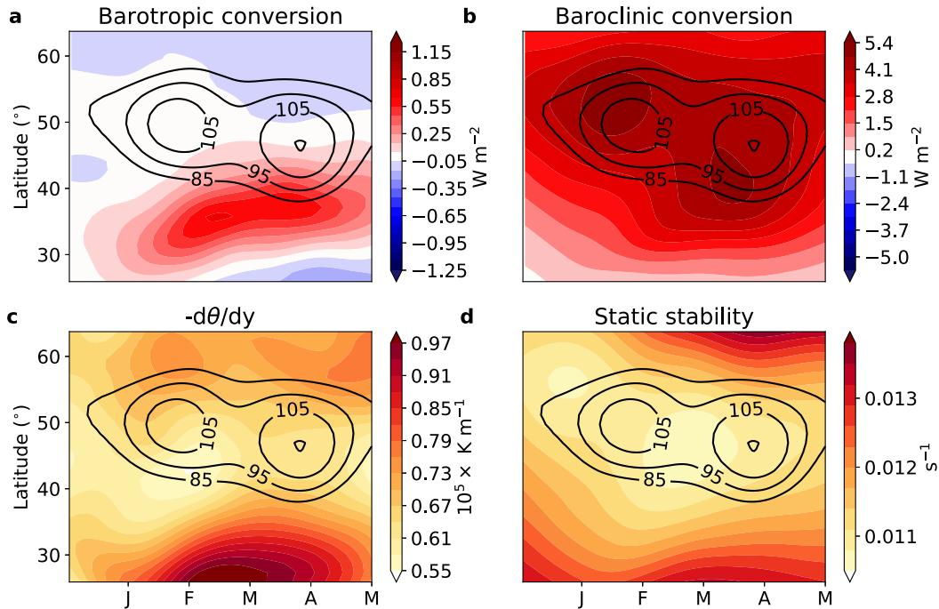
FIG. 5. Seasonality of the conversion terms in the Lorenz energy cycle from the control run (oc10qf40). (a) Vertically integrated barotropic conversion from mean to eddy kinetic energy. (b) Vertically integrated baroclinic conversion from mean to eddy potential energy. (c) Meridional potential temperature gradient (850 hPa). (d) Static stability (850 hPa). The black contours show the meridional velocity variance  $v^2$  at  $\sigma = 0.37$  for 2–6.5-day eddies, as in Fig. 4b.
