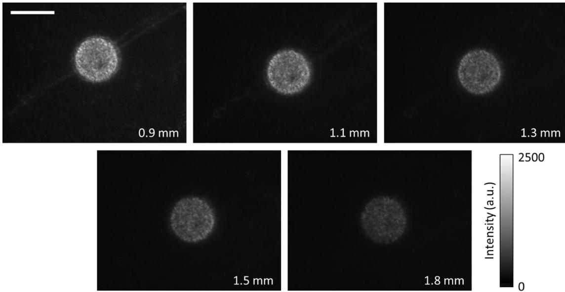
**Fig. S1. Dark-field images of a 50- $\mu$ m-diameter polystyrene bead in water with various beam block diameters.**
