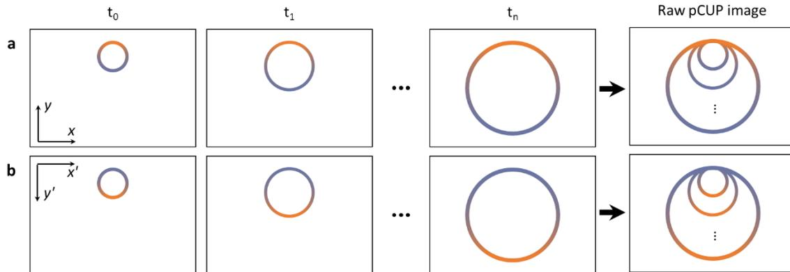
**Fig. S2. Illustration of the raw image formation with 180° rotated complementary views.** (a) The original pCUP raw image formation without a 180° rotation. The signals from the top half of the shockwave (shown in orange) are overlapped in the raw image. (b) The raw image formation with a 180° rotation. The bottom half (shown in blue) is placed at the top of the image and experiences the overlap of signals.
