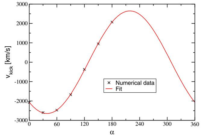
FIG. 3. The recoil velocity computed numerically from the GW signal for  $p = 0.075$  is shown as  $\times$  symbols for different values of the spin orientation  $\alpha$ . The red curve represents the fit obtained from these data according to Eq. (3). Only data for  $\alpha < 180^\circ$  are needed to determine the fitting coefficients, due to the symmetry of the superkick configurations.
