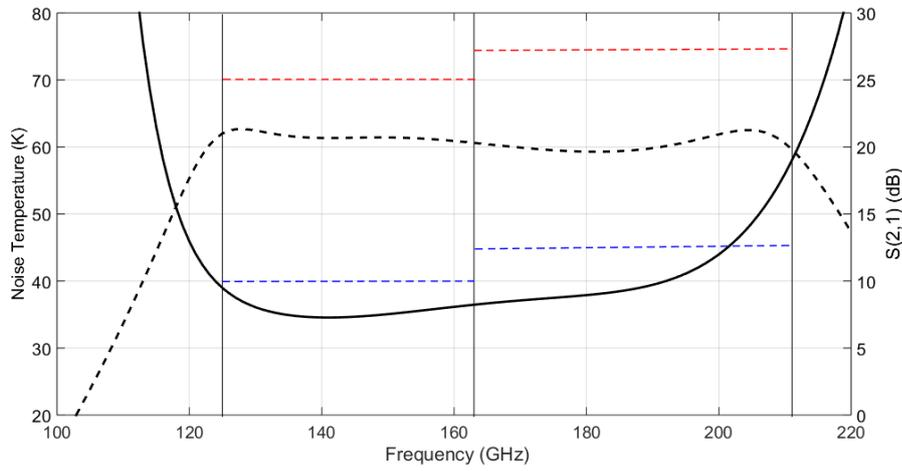
**Fig. 2** Noise Temperature (solid) and Forward Transmission (dotted) simulated results. Dotted blue and red lines indicate the 80 and 100 % noise temperature LNA specifications, respectively, for each sub-band.
